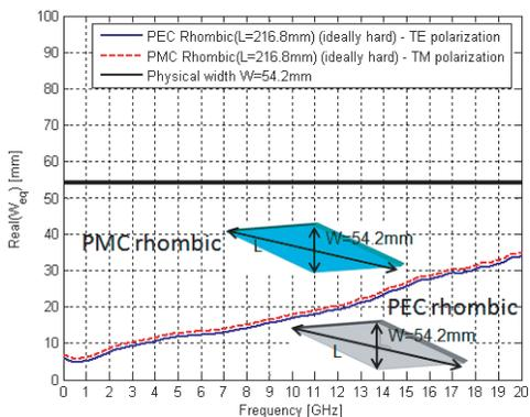
**Figure 4.** Equivalent blockage width of ideally PEC and PMC rhombic cross-section under normal incidence ( $\varphi = 0^\circ$ ).
