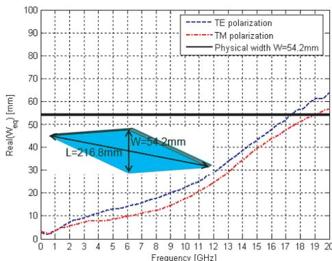
**Figure 10.** Equivalent blockage width of ideally PMC hard strut with narrow metallic strips ( $p = 6\text{ mm}$  and  $s = 3\text{ mm}$ ) under normal incidence ( $\varphi = 0^\circ$ ).
