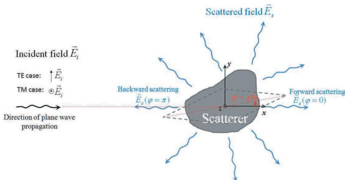
**Figure 1.** Plane wave scattering (2D case).
