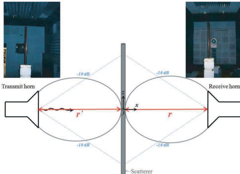
**Figure 14.** Measurement setup for measuring blockage width of scatterers in the anechoic chamber at Universidad Politécnica de Madrid.
