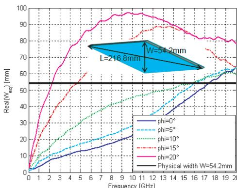
**Figure 11.** Equivalent blockage width of a ideally PMC hard strut with narrow metallic strips ( $p = 6\text{ mm}$  and  $s = 3\text{ mm}$ ) under variation of  $\varphi$  for TE case.
