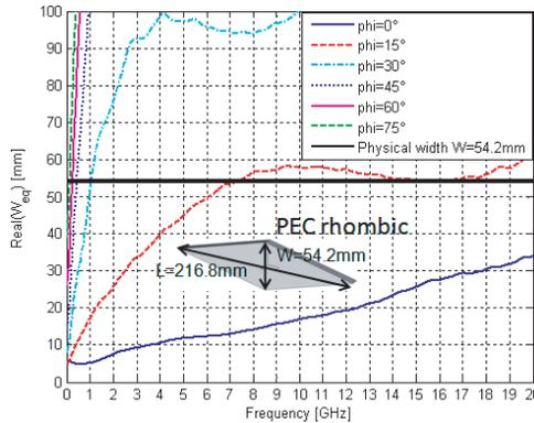
**Figure 5.** Equivalent blockage width of PEC rhombus under variation of  $\varphi$  in the azimuth plane for TE polarization.
