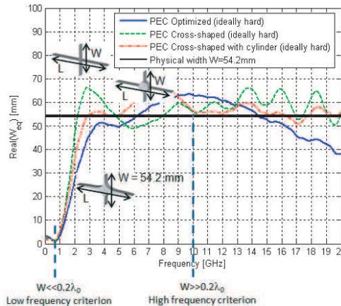
**Figure 3.** Equivalent blockage width of ideally hard cross-shaped sections (width  $W$ , length  $L = 2W$ ) under normal incidence ( $\varphi = 0^\circ$ ).
