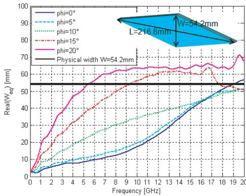
**Figure 12.** Equivalent blockage width of a ideally PMC hard strut with narrow metallic strips ( $p = 6$  mm and  $s = 3$  mm) under variation of  $\varphi$  for TM case.
