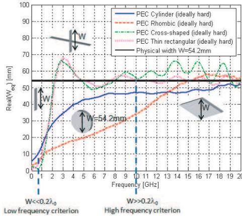
**Figure 2.** Equivalent blockage width for TE case of ideally hard cylinders with different cross-sectional shapes (basic-shaped cross sections) under normal incidence ( $\varphi = 0^\circ$ ).
