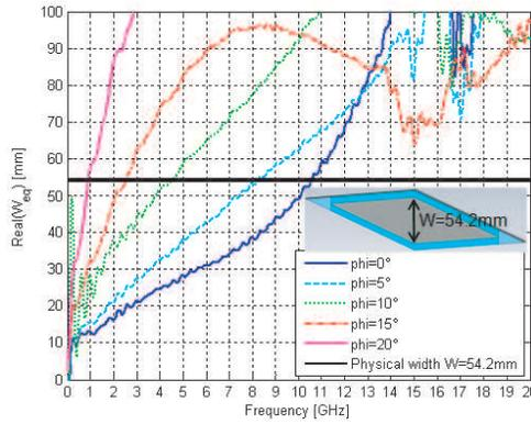
**Figure 8.** Equivalent blockage cross section of strip-loaded dielectric coated metal strut when the strip period  $p = 6$  mm and the strip width  $s = 3$  mm under variation of  $\varphi$  in the azimuth plane for TE polarization.
