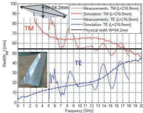
**Figure 13.** Equivalent blockage width for simulated model — prototype: ideal PEC rhombic cross section strut of  $W = 54.2$  mm and  $L = 216.8$  mm under normal incidence ( $\varphi = 0^\circ$ ).
