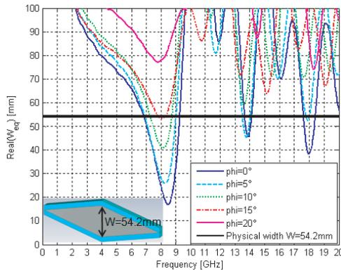
**Figure 6.** Equivalent blockage width of PEC rhombus with dielectric coating  $\epsilon_r = 2.2$  under variation of  $\varphi$  in the azimuth plane for TM polarization.
