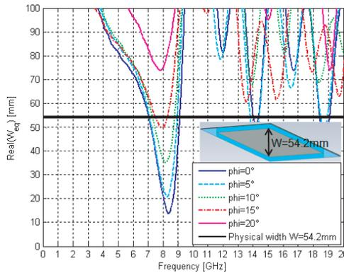
**Figure 9.** Equivalent blockage cross section of strip-loaded dielectric coated metal strut when the strip period  $p = 6$  mm and the strip width  $s = 3$  mm under variation of  $\varphi$  in the azimuth plane for TM polarization.
