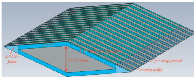
**Figure 7.** Cross section detail of strip-loaded dielectric coated metal strut: strip period  $p$  and strip width  $s$ .
