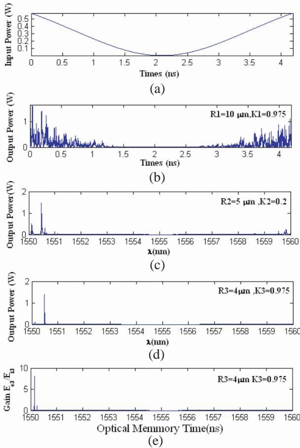
**Figure 12.** Simulation results obtained when a dark soliton pulse is input into a micro and nanoring resonator system, where the parameters used are (a)  $R_1 = 10 \mu\text{m}$ ,  $R_2 = 5 \mu\text{m}$ ,  $R_3 = 2.5 \mu\text{m}$ , center wavelength at 1,550 nm, and (b)  $R_1 = 10 \mu\text{m}$ ,  $R_2 = 5 \mu\text{m}$ ,  $R_3 = 4 \mu\text{m}$ , center wavelength at 1,550 nm and  $\kappa_1 = \kappa_3 = 0.975$ ,  $\kappa_2 = 0.2$ , with 20,000 roundtrips.
