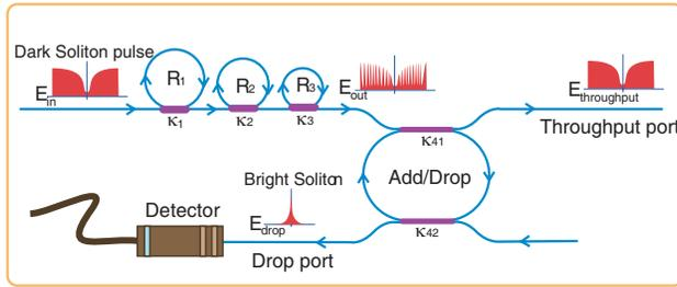
**Figure 4.** A schematic of a dark-bright soliton conversion system, where  $R_s$ : Ring radii,  $\kappa_s$ : Coupling coefficients,  $\kappa_{41}$  and  $\kappa_{42}$  are the add/drop coupling coefficients.
