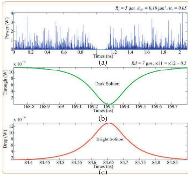
**Figure 6.** Simulation results of the optical solitons, where (a) the signals in  $R_3$ , (b) a dark soliton and (c) a bright soliton. The input dark soliton power is  $0.65 \text{ W}$ ,  $\kappa_1 = 0.5$ ,  $R_d = 10 \mu\text{m}$ .
