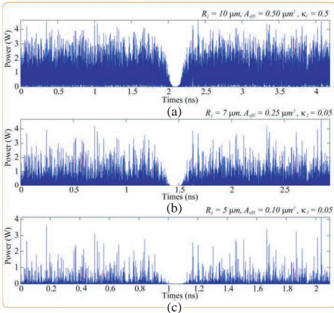
**Figure 5.** Simulation results of the soliton signals within the ring resonator system, where (a) in ring  $R_1$ , (b) in ring  $R_2$  and (c) in ring  $R_3$ .
