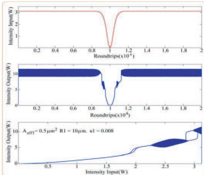
**Figure 2.** Simulation results obtained when a dark soliton pulse is input into a microring resonator, where  $R_1 = 10 \mu\text{m}$ ,  $A_{eff1} = 0.50 \mu\text{m}^2$ ,  $\kappa_1 = 0.009$ .
