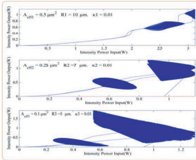
**Figure 3.** Simulation results of a dark soliton pulse propagating in a microring resonator system, where  $R_1 = 10 \mu\text{m}$ ,  $A_{eff1} = 0.50 \mu\text{m}^2$ ,  $R_2 = 7 \mu\text{m}$ ,  $A_{eff2} = 0.25 \mu\text{m}^2$ ,  $R_3 = 5 \mu\text{m}$ ,  $A_{eff3} = 0.10 \mu\text{m}^2$ ,  $\kappa_1 = 0.01$  and  $\kappa_2 = \kappa_3 = 0.01$ .
