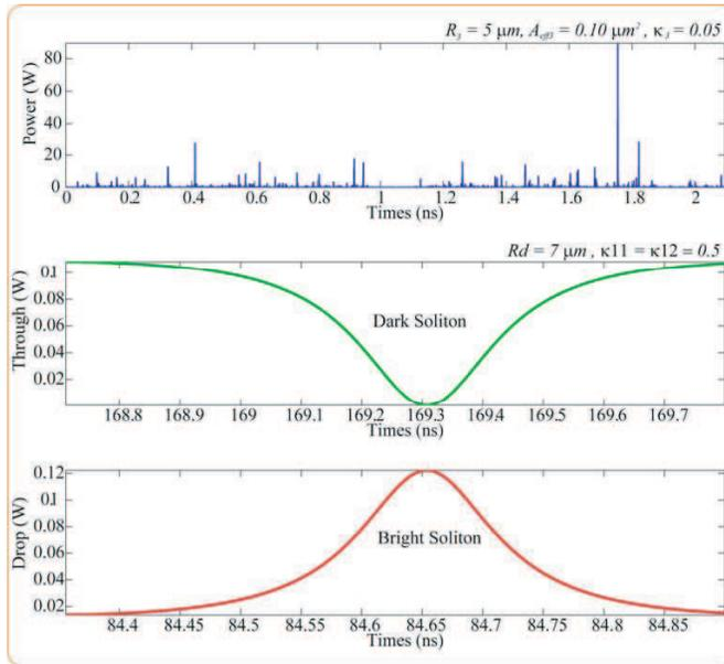
**Figure 7.** Simulation results of the optical solitons, where (a) the signals in  $R_3$ , (b) a dark soliton and (c) a bright soliton. The input dark soliton power is 0.65 W,  $\kappa_1 = 0.9$ ,  $R_d = 10 \mu\text{m}$ .
