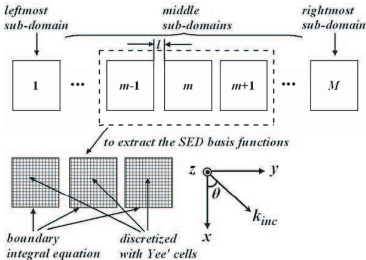
**Figure 1.** The  $M$  elements are included in the  $M$  sub-domains, whose boundaries are close to the elements. Three adjacent sub-domains are separated from the  $M$  sub-domains in order to extract the SED basis functions for the whole grating. They are discretized with Yee's cells, and a boundary integral equation is set up on their boundaries.
