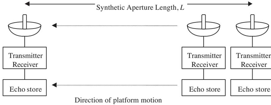
**Figure 2.2.** Synthetic aperture.
