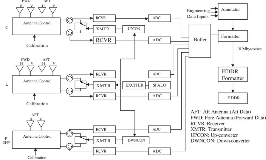
**Figure 1.2.** NASA/JPL aircraft imaging radar functional diagram.
