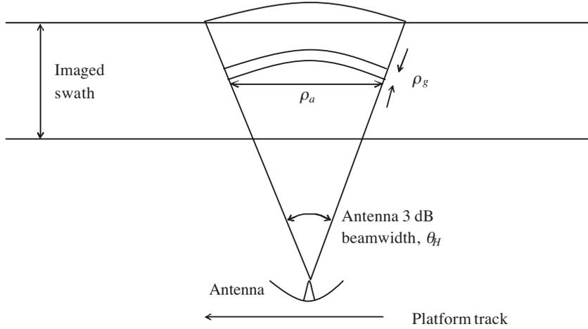
**Figure 2.5.** Azimuth resolution of a RAR.
