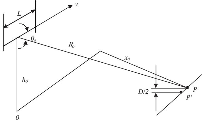
**Figure 2.6.** Illustration of azimuth resolution of SAR.
