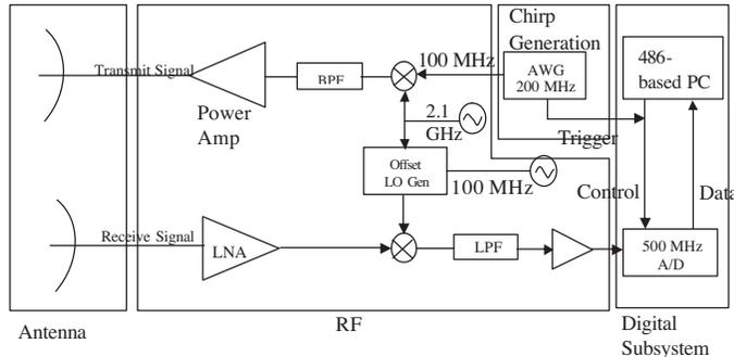
**Figure 1.3.** YSAR block diagram.
