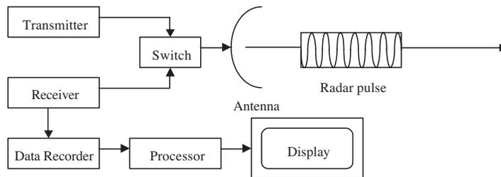
**Figure 2.1.** Basic block diagram of typical radar system.
