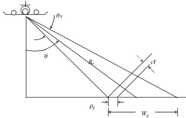
**Figure 2.4.** Range resolution of a real aperture radar.
