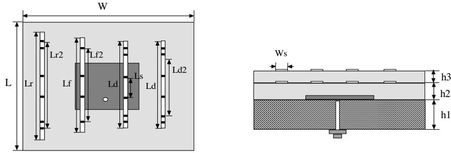
**Figure 10.** Parameters of antenna with a Yagi-Uda substrate cover.
