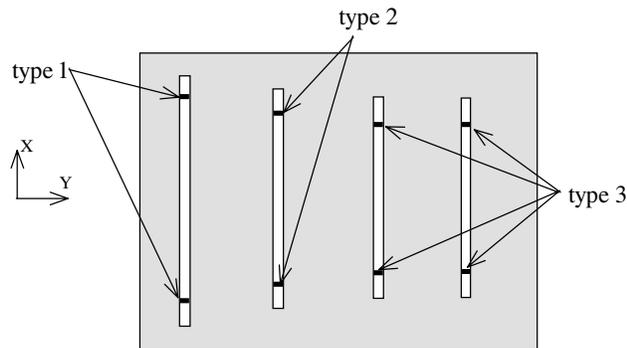
**Figure 6.** Structure of reconfigurable Yagi-Uda substrate.
