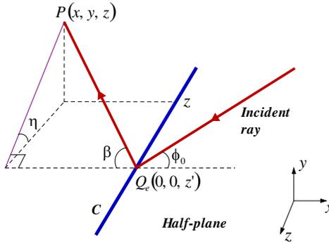
**Figure 2.** General geometry for the edge diffraction.
