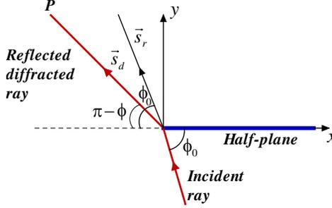
**Figure 4.** Diffraction geometry for the reflected diffracted waves.
