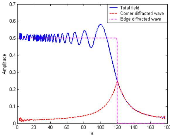
**Figure 8.** Compensation of the edge diffracted wave.
