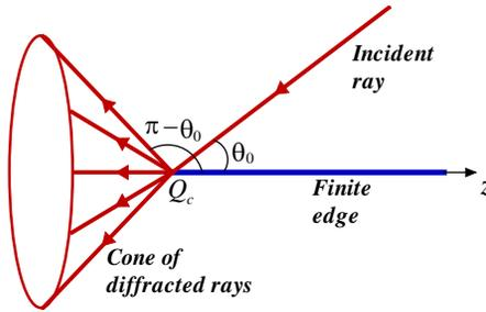
**Figure 6.** Discontinuity of the edge diffracted wave.
