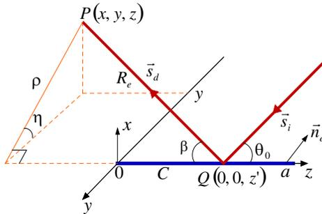
Figure 5. Geometry of the finite edge.
