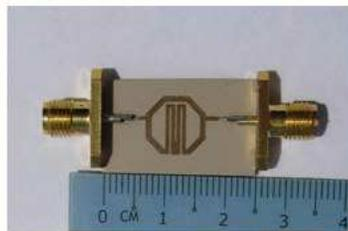
**Figure 9.** The top view of the fabricated dual-mode bandpass filter.
