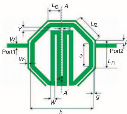
**Figure 3.** Compressed dual-mode microstrip bandpass filter.
