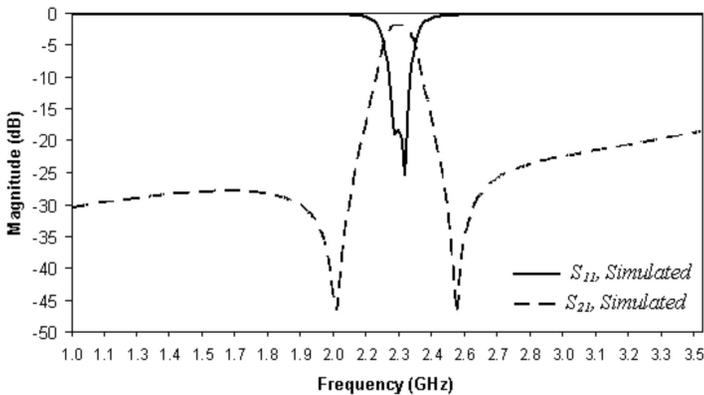
**Figure 7.** The simulation results for proposed dual-mode filter.
