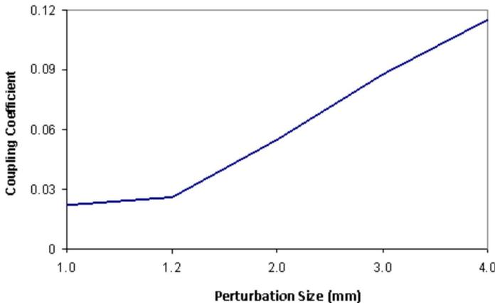
**Figure 6.** Simulated coupling coefficient versus the size of perturbation.
