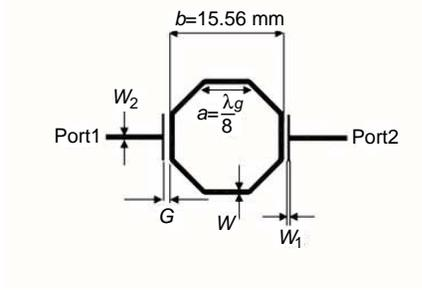
**Figure 1.** Single mode octagonal ring resonator.
