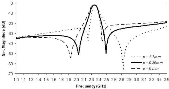
**Figure 4.** Variation of the filter frequency response for different tab position of feedlines.
