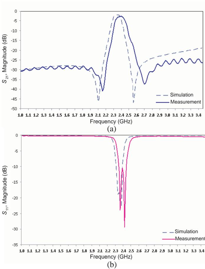
**Figure 8.** (a) The simulated and measured  $S_{21}$  frequency responses of the Filter. (b) The simulated and measured  $S_{11}$  frequency responses of the filter.
