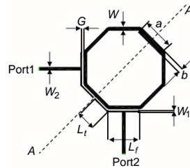
**Figure 2.** Conventional structure of dual-mode bandpass filter [6].
