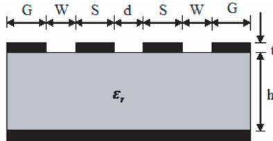
**Figure 2.** Cross section of conductor-backed edge-coupled CPW.
