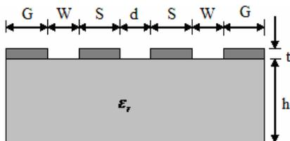
**Figure 1.** Cross section of edge coupled coplanar waveguides.
