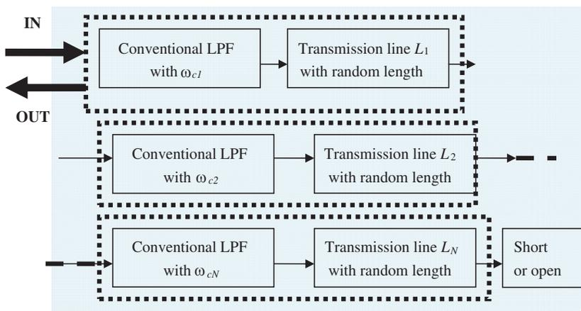
**Figure 3.** The scheme map of the compressive sensing filter by LPF.
