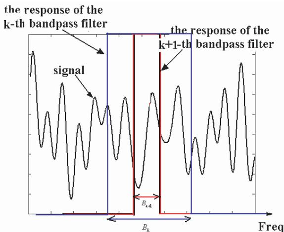
**Figure 2.** The illustration of CSF based on the ideal conventional band-pass filter.
