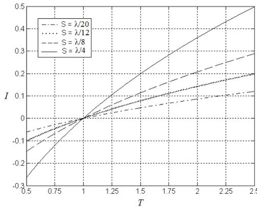
**Figure 8.** Amplitude of reflection coefficient versus  $T$  for three values of  $S$ .  $\lambda$  is the wave length of an unloaded line (i.e.,  $I = 0$ ).
