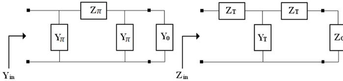
**Figure 4.** Isolated symmetrical  $\pi$  or T cell between transmission lines.
