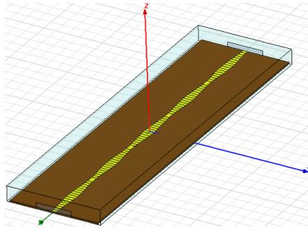
Figure 14. HFSS scheme of the periodic structure.
