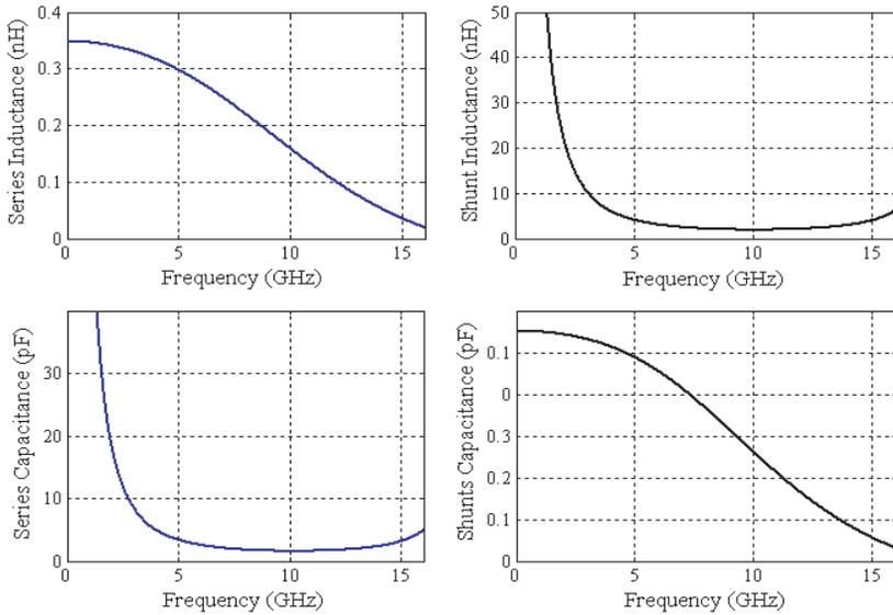
**Figure 13.** Series and shunt inductances and capacitances shown in two possible equivalent circuits in Figure 12.
