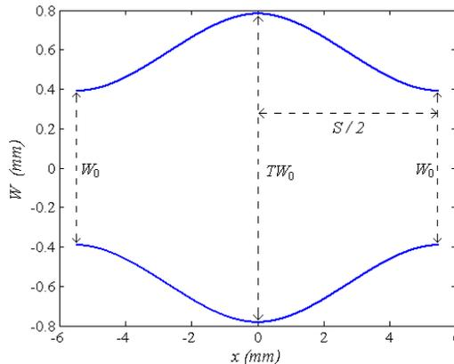
**Figure 7.** The geometry of proposed symmetrical microstrip cell.
