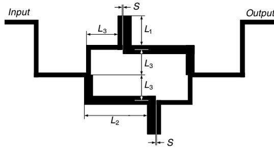
**Figure 8.** CCDBR filter: geometry [32].
