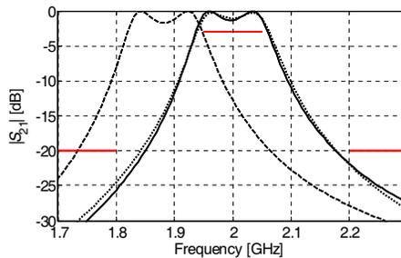
**Figure 7.** Bandpass filter with open stub inverter:  $\mathbf{R}_f$  response (solid line) at the final design obtained after two iterations of our optimization procedure; fine (dashed line) and coarse (dotted line) model responses at the initial design.
