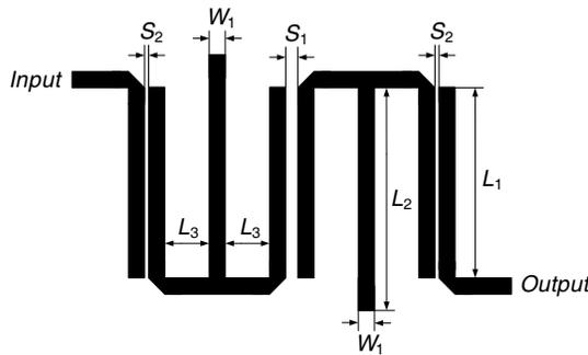
**Figure 5.** Bandpass filter with open stub inverter: geometry [31].
