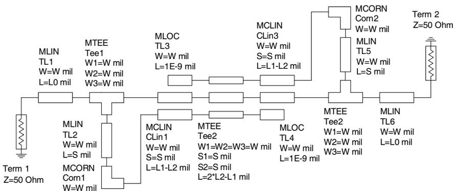
Figure 3. DFS filter: coarse model (Agilent ADS).
