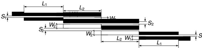
**Figure 10.** Third-order Chebyshev bandpass filter: geometry [34].
