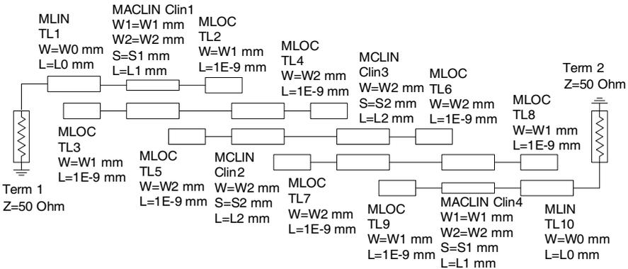
**Figure 11.** Third-order Chebyshev filter: coarse model (Agilent ADS).
