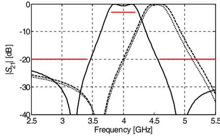
**Figure 9.** CCDBR filter: fine model response (solid line) at the final design obtained after two iterations of the proposed optimization procedure; fine (dashed line) and coarse (dotted line) model responses at the initial design.
