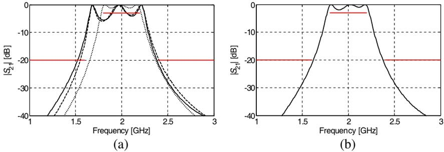
**Figure 12.** Third-order Chebyshev filter: (a) fine (solid line) and coarse (dotted line) model responses at the initial design  $\mathbf{x}^{(0)}$  and the coarse model response (dashed line) design at  $\mathbf{x}_c^{(0)}$ ; (b) fine model response (solid line) at the design obtained after two iterations of our generalized optimization procedure.
