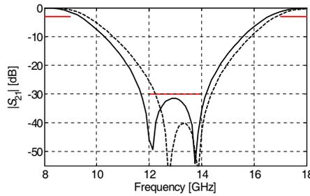
**Figure 4.** DFS filter: fine (solid line) and coarse (dashed line) model responses at the design obtained after one iteration of the proposed optimization procedure.
