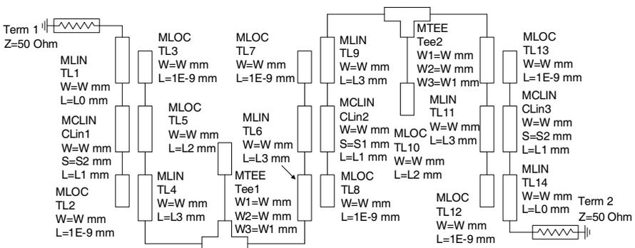
**Figure 6.** Bandpass filter with open stub inverter: coarse model (Agilent ADS).
