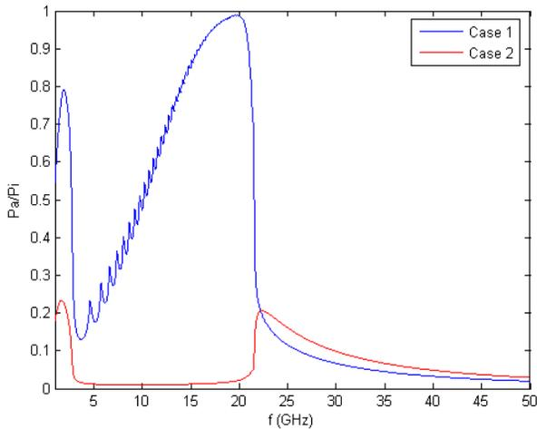
**Figure 9.** Normalized absorbed power comparison for linearly increasing (case 1) and decreasing profiles (case 2).  $\nu_{en} = 1$  GHz,  $N_m = 5 \times 10^{18} \text{ m}^{-3}$ ,  $B = 0.1$  T.
