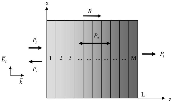
**Figure 1.** Electromagnetic wave propagation through a plasma layer with equi-width subslabs.
