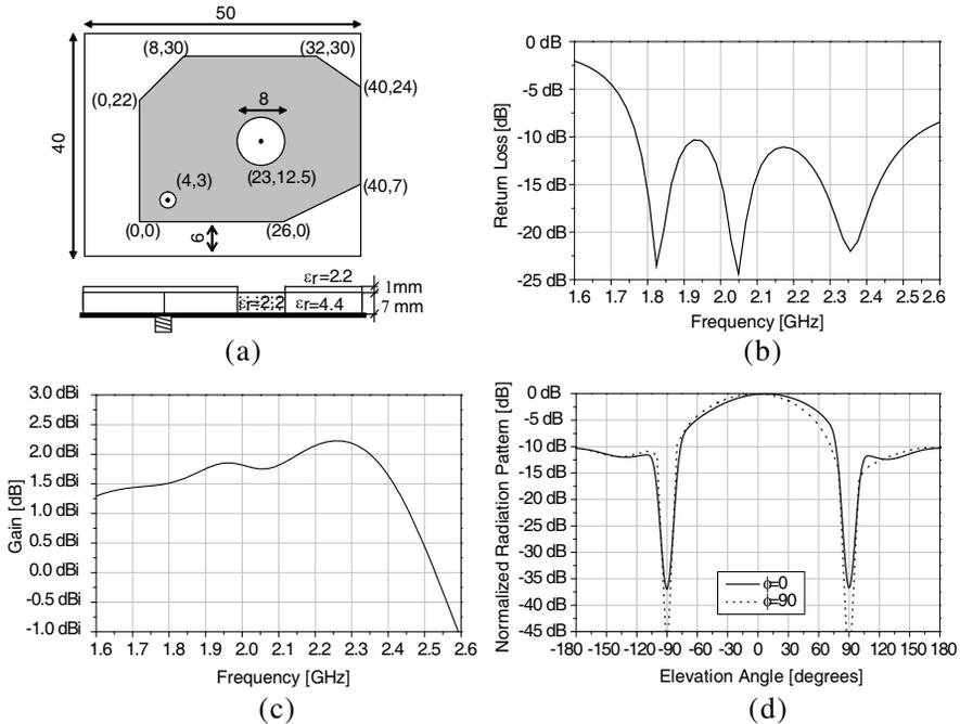
**Figure 7.** (a) Layout of a polygonal patch antenna with a circular slot for the operation in GSM, PCS, UMTS, Wi-Fi, and Bluetooth frequency bands. (b) Return loss as a function of frequency. (c) Gain as a function of frequency. (d) Polar radiation patterns at the central frequency of the UMTS service (2050 MHz) on both the principal planes.
