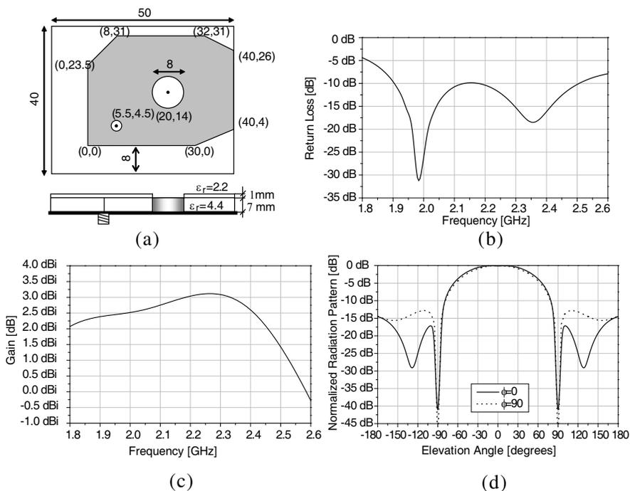
**Figure 6.** (a) Layout of a polygonal patch antenna with a circular slot for the operation in UMTS, Wi-Fi, and Bluetooth frequency bands. (b) Return loss as a function of frequency. (c) Gain as a function of frequency. (d) Polar radiation patterns at the central frequency of the UMTS service (2050 MHz) on both the principal planes.
