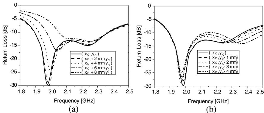
**Figure 3.** Effects of the insertion of a shorting post on the fundamental modes of the antenna depicted in Fig. 1(a). (a) Simulated return loss as a function of the frequency for different positions of the shorting post along the  $x$ -axis. (b) Simulated return loss as a function of the frequency for different positions of the shorting post along the  $y$ -axis.
