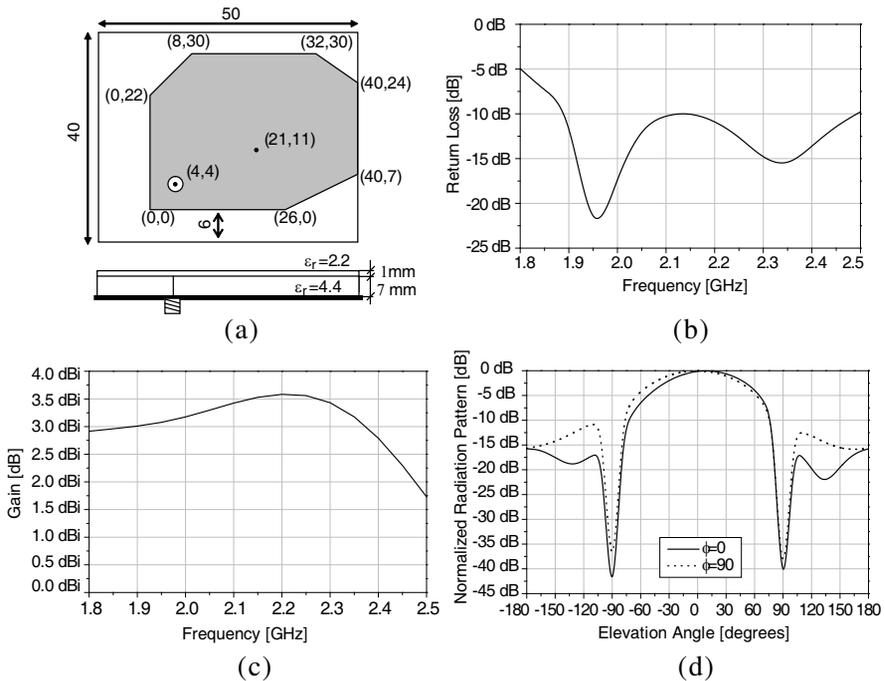
**Figure 4.** (a) Layout of a polygonal patch antenna with a shorting post for the operation in UMTS, Wi-Fi, and Bluetooth frequency bands. (b) Return loss as a function of frequency. (c) Gain as a function of frequency. (d) Polar radiation patterns at the central frequency of the UMTS service (2050 MHz) on both the principal planes.
