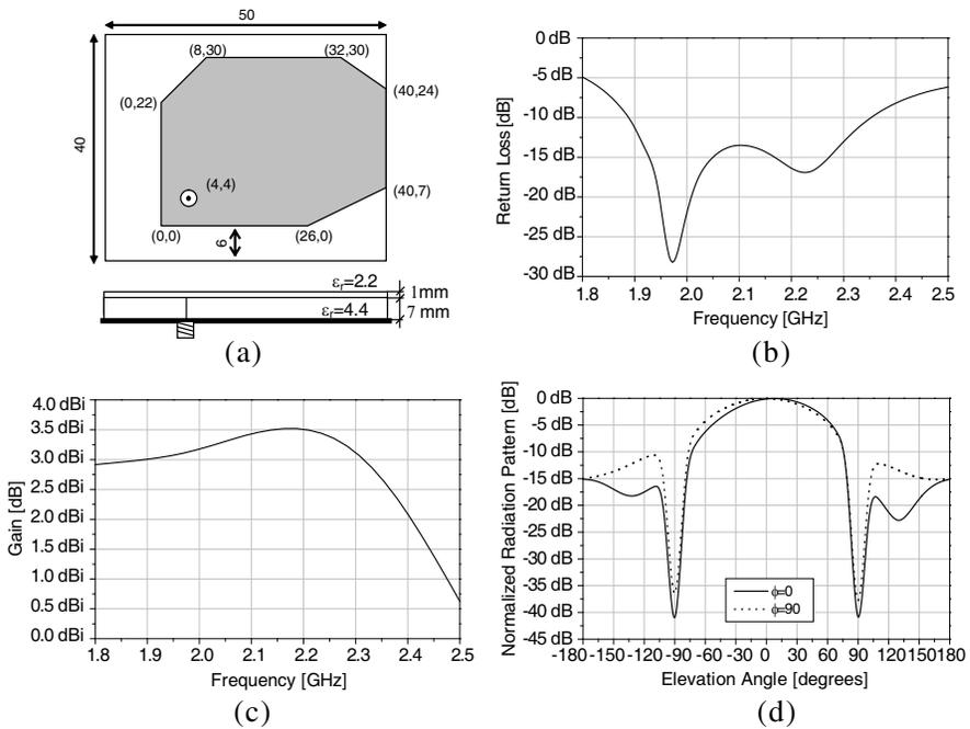
**Figure 1.** (a) Polygonal patch antenna layout for UMTS terminals, and (b) its impedance, (c) gain and (d) radiating features at the central UMTS frequency of 2050 MHz. The antenna is fed by a  $50 \Omega$  coaxial probe and is covered by a plastic overlay. The geometrical dimensions in Fig. 1(a) are expressed in mm. The results presented in this figure come from [23].
