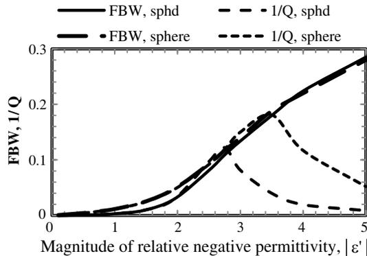
**Figure 5.** Fractional conductance bandwidth  $FBW_{cd}$  (FBW (32),  $1/Q$  (37), (38)) ( $\beta = 1$ ) of the oblate spheroidal (sphd) and spherical (sphere) antennas in the shells as functions of magnitude of the negative real part of relative permittivity  $|\epsilon'|$ .
