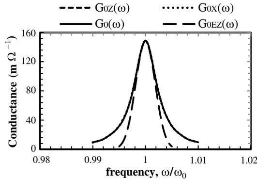
**Figure 3.**  $G_0(\omega)$  — conductance of the oblate spheroidal antenna in the shell with relative permittivity  $\varepsilon = -1 - 0.004i$  tuned on resonance at frequency  $\omega_0$  (2),  $G_{0z}(\omega)$  — approximation of  $G_0(\omega)$  with parameter  $Z'_0(\omega_0)$  (19),  $G_{0x}(\omega)$  — approximation of  $G_0(\omega)$  with  $X'_0(\omega_0)$  (20),  $G_{0EZ}(\omega)$  — approximation of  $G_0(\omega)$  with  $Z'_0(\omega_0)$  (21).
