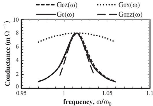
**Figure 4.**  $G_0(\omega)$  — conductance of the of the oblate spheroidal antenna in the shell with relative permittivity  $\epsilon = -2.05 - 0.004i$  tuned on resonance at frequency  $\omega_0$  (2),  $G_{0Z}(\omega)$  — approximation of  $G_0(\omega)$  with parameter  $Z'_0(\omega_0)$  (19),  $G_{0X}(\omega)$  — approximation of  $G_0(\omega)$  with  $X'_0(\omega_0)$  (20),  $G_{0EZ}(\omega)$  — exponential approximation of  $G_0(\omega)$  with  $Z'_0(\omega_0)$  (21).
