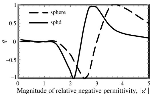
**Figure 2.** Parameter of antiresonant conditions  $q = \frac{R'_0(\omega_0)}{|Z'_0(\omega_0)|}$  for the oblate spheroidal and spherical antennas in the shells as functions of magnitude of the real part of relative negative permittivity  $|\epsilon'|$ .
