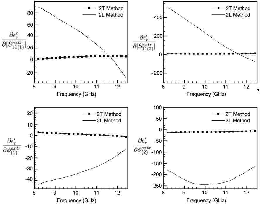
**Figure 2.**  $\epsilon_r'$  amplification factors computed for the two-thickness method (2T Method) and the two-layer method (2L Method) using one layer of FGM-125 as measurement 1 and two layers of FGM-125 as measurement 2.
