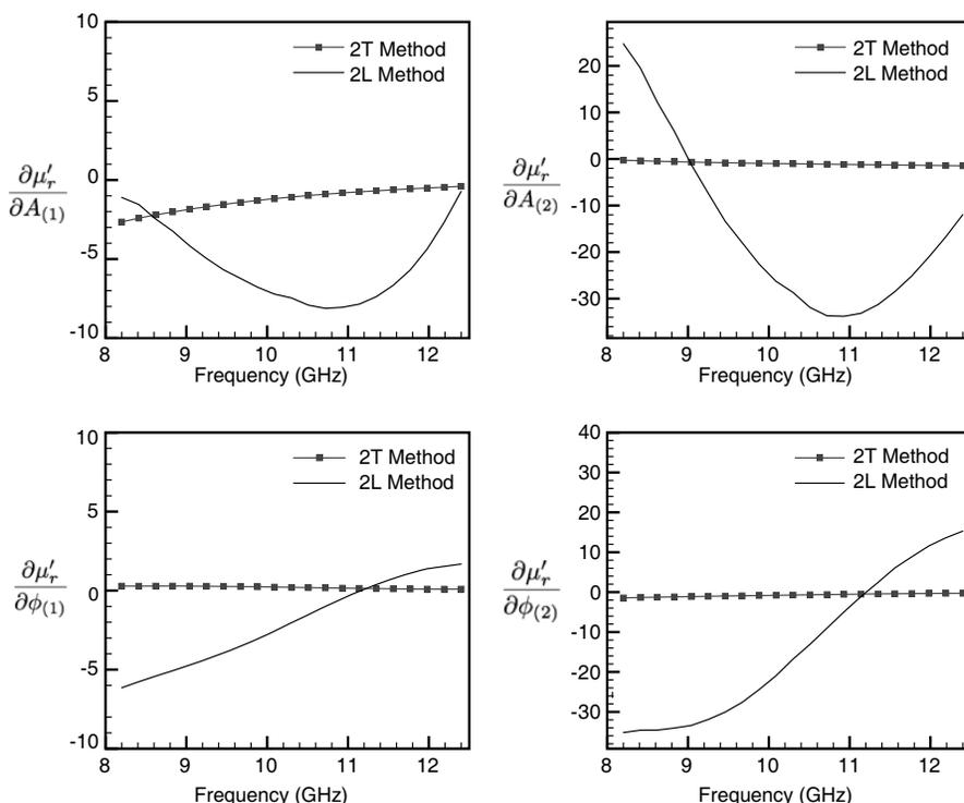
**Figure 3.**  $\mu'_r$  amplification factors computed for the two-thickness method (2T Method) and the two-layer method (2L Method) using one layer of FGM-125 as measurement 1 and two layers of FGM-125 as measurement 2.
