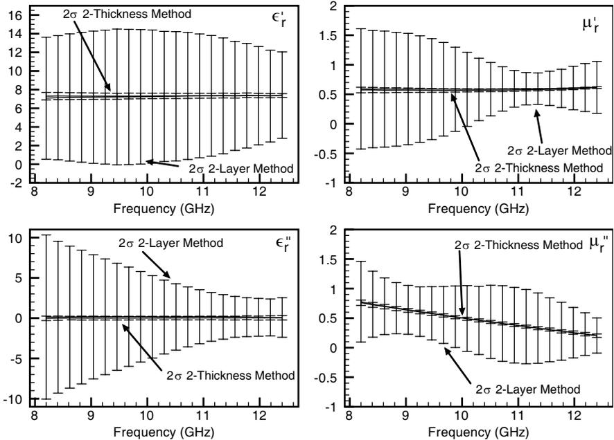
**Figure 4.** Errors due to VNA measurement uncertainty using the two-layer and two-thickness methods for ECCOSORB<sup>®</sup> FGM-125. Error bars show  $\pm 2\sigma$ .
