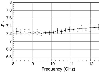
**Figure 7.** Extracted  $\epsilon'_r$  for FGM-125 using the two-thickness method.
