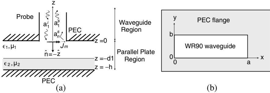
**Figure 1.** (a) Side view and (b) top view for two layers of material interrogated by a single waveguide probe.
