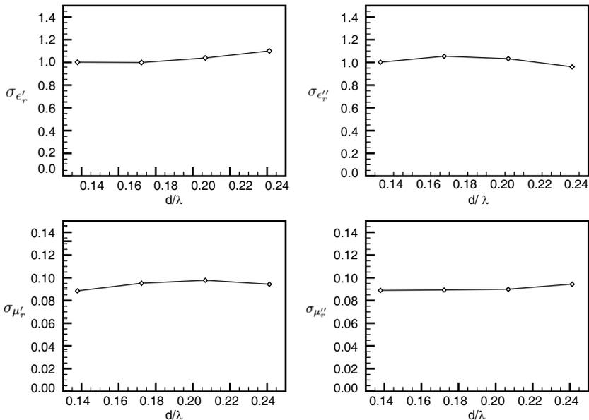
**Figure 6.** Errors due to VNA measurement uncertainty using the two-layer method for ECCOSORB<sup>®</sup> FGM-125. The known-material layers are plexiglass with various thicknesses.
