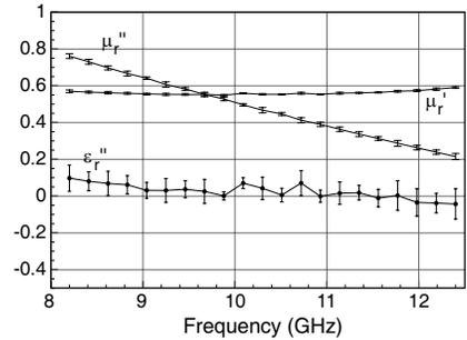
**Figure 8.** Extracted material parameters for a FGM-125 using the two-thickness method.
