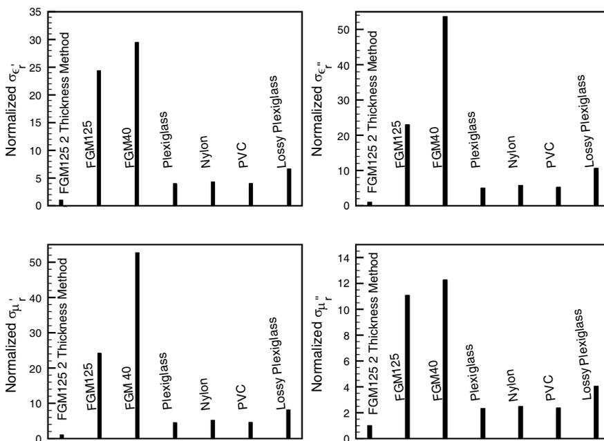
**Figure 5.** Errors due to VNA measurement uncertainty using the two-layer method for ECCOSORB<sup>®</sup> FGM-125 at 10.09 GHz. Bars show the standard deviation for several known-material layers normalized to the standard deviation found using the two-thickness method. Known-material layer thicknesses in inches/mm are: 0.125/3.175 (FGM-125), 0.04/1.016 (FGM-40), 0.125/3.175 (Plexiglass and “lossy Plexiglass”), 0.125/3.175 (Nylon), 0.119/3.023 (PVC).
