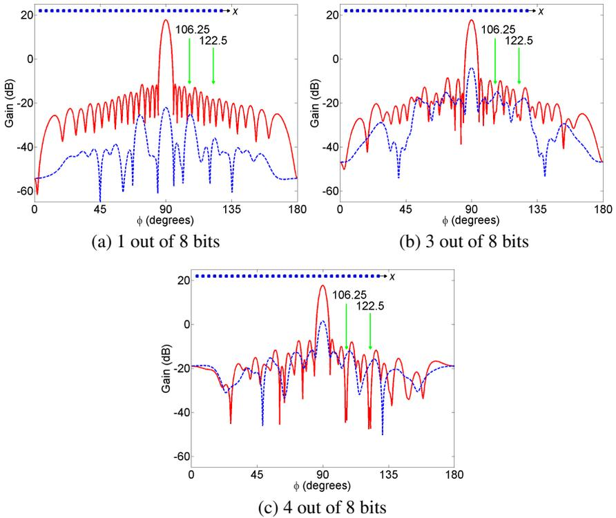
**Figure 5.** Phase only nulling with the dipole array and limits on the phase quantization. The adapted pattern is the solid line and the cancellation pattern is the dashed line.
