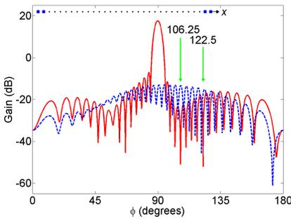
**Figure 13.** Amplitude and phase adaptive nulling using 4 edge elements. The adapted pattern is the solid line and the cancellation pattern is the dashed line.
