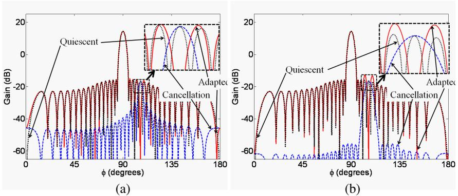
**Figure 1.** Null placed at  $\phi = 106.25^\circ$  in 30 dB  $\bar{n} = 7$  Taylor quiescent pattern with cancellation patterns that are (a) uniform  $c_n = 1.0$  (b) tapered  $c_n = a_n$ .
