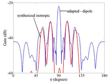
**Figure 7.** Adaptive cancellation pattern from the 32 element dipole array compared to the synthesized cancellation pattern of the 32 element array of isotropic point sources.
