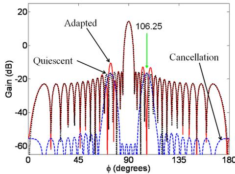
**Figure 2.** The cancellation pattern (dashed line) superimposed on the quiescent pattern and adapted pattern when a null is placed at  $\phi = 106.25^\circ$  using phase weights and  $c_n = a_n$ .
