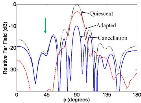
**Figure 15.** Plots of the experimental quiescent and adapted patterns for a null at  $45^\circ$ . The plot of the cancellation pattern is the difference between the adapted and quiescent patterns.
