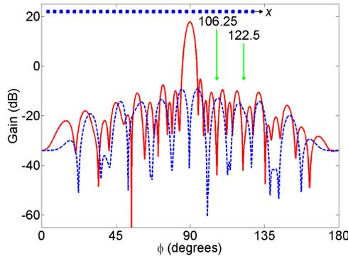
**Figure 8.** Adapted pattern with interference at  $\phi = 106.25^\circ$  and  $122.5^\circ$  and superimposed on the quiescent pattern. Symmetric elements receive bitwise complements of the 4 out of 8 adaptive phase bits in order to minimize the cancellation pattern peak at  $\phi = 90^\circ$ . The adapted pattern is the solid line and the cancellation pattern is the dashed line.
