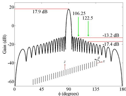
**Figure 4.** 32 element array of dipoles along the  $x$ -axis Quiescent pattern of the 32 element low sidelobe dipole array.
