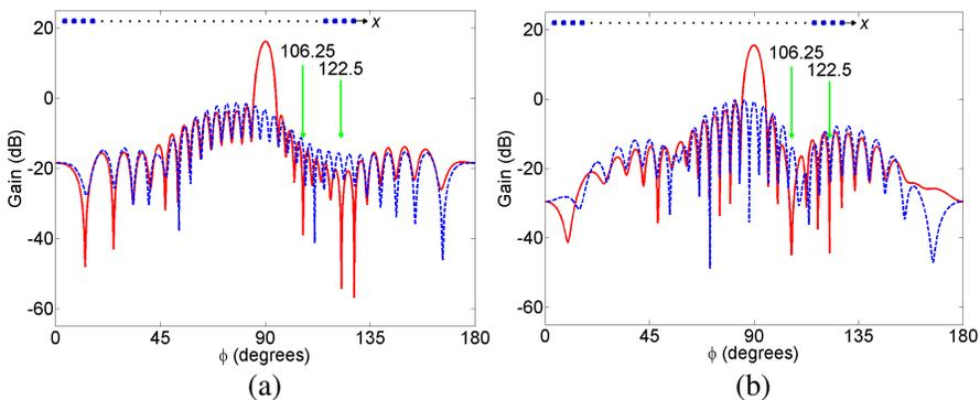
**Figure 10.** Adapted, quiescent, and cancellation patterns for the 32 element dipole array when elements 1, 2, 3, 4, 29, 30, 31, and 32 are adaptive (a) phase-only (b) amplitude and phase. The adapted pattern is the solid line and the cancellation pattern is the dashed line.
