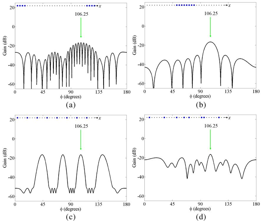
**Figure 3.** Cancellation patterns for 4 different selections of adaptive elements that place a null at  $\phi = 106.25^\circ$ . The array at the top of the plots shows a diagram of the linear array along the  $x$ -axis. Adaptive elements are indicated by large squares. (a) adaptive elements: 1, 2, 3, 4, 29, 30, 31, 32; (b) adaptive elements: 13, 14, 15, 16, 17, 18, 19, 20; (c) adaptive elements: 1, 5, 9, 13, 17, 21, 25, 29; (d) adaptive elements: 2, 8, 13, 16, 18, 23, 24, 30.
