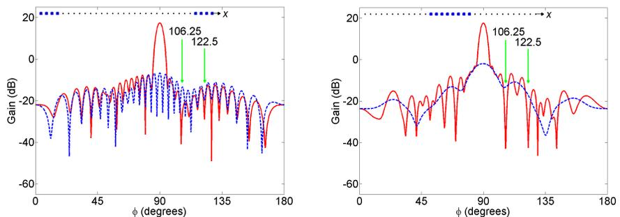
**Figure 11.** Results for the case in Fig. 10(a) when the adapted phase is limited to  $90^\circ$ . The adapted pattern is the solid line and the cancellation pattern is the dashed line.
