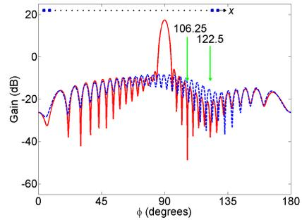
**Figure 14.** Phase-only adaptive nulling using 4 edge elements. The adapted pattern is the solid line and the cancellation pattern is the dashed line.
