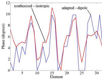
**Figure 6.** Adaptive phase (phase-only nulling with 3 bits) from 32 element dipole array compared to the synthesized phase of the 32 element array of isotropic point sources.
