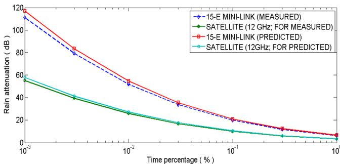
**Figure 3.** Comparison of terrestrial and satellite rain attenuation.
