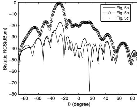
**Figure 6.** The bistatic RCSs for a 3D cloak in three layered media when the plane wave is incident obliquely.
