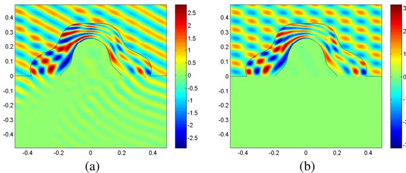
**Figure 3.** (color online) The real parts of the electric fields  $E_x$  for half of a 3D cloak in the upper half space (air) and lower half space (earth medium) when the plane wave is incident obliquely. (a) The earth medium is lossy medium with  $\epsilon_{r2} = 2 - j0.2$ . (b) The earth medium is PEC.
