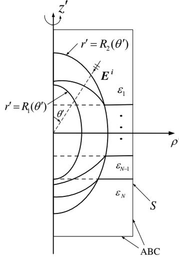
**Figure 1.** The slice of a 3D cloak embedded in  $N$ -layered media with ABC. The cloaking shell exists in the region defined by  $R_1(\theta') < r' < R_2(\theta')$ . The layer interfaces inside the cloak become curves described by (17).
