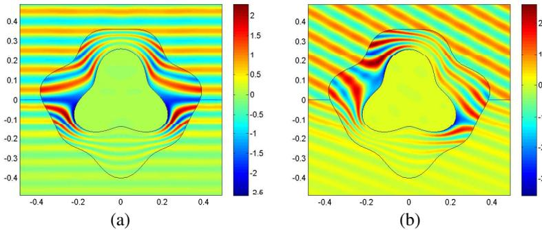
**Figure 2.** (color online) The real parts of the electric fields  $E_x$  for a 3D cloak in the  $xoz$  plane when the plane wave is illuminated. (a) The incident angle is  $0^\circ$ . (b) The incident angle is  $30^\circ$ .
