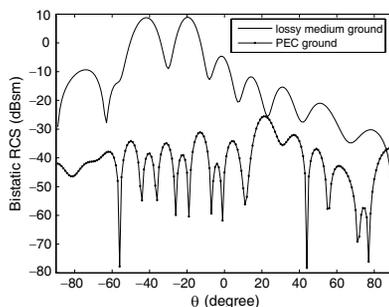
**Figure 4.** The bistatic RCSs for half of a 3D cloak in the upper half space (air) and lower half space (earth medium) when the plane wave is incident obliquely.
