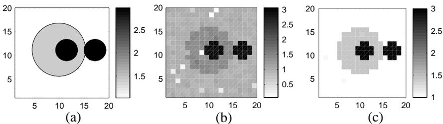
**Figure 5.** Reconstructions of **FoamTwinDiel**. (a) Original object. Reconstruction using: (b) Standard PSO, (c) PSO-SA-TS.
