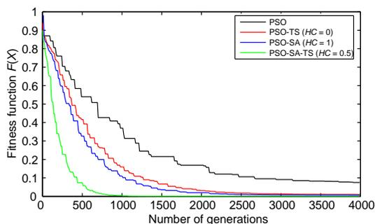
**Figure 4.** Fitness function  $F$  at different generations in inversion of **FoamDielExt** using both hybrid algorithms and standard PSO.
