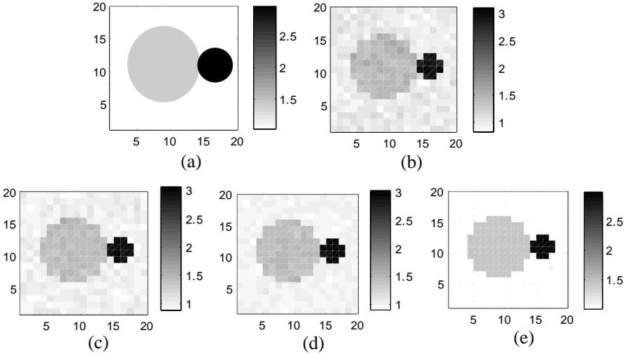
**Figure 3.** Reconstructions of the **FoamDielExt**. (a) Original object. (b) Reconstruction using standard PSO. Reconstruction for different value of  $HC$ , (c)  $HC = 0$ , (d)  $HC = 1$  and (e)  $HC = 0.5$ .
