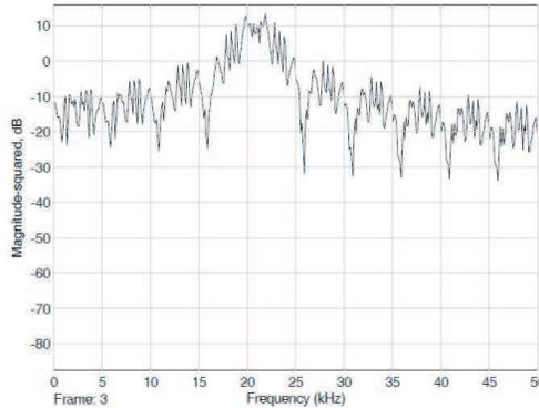
**Figure 5.** Power spectral density of IF signal before correlation.
