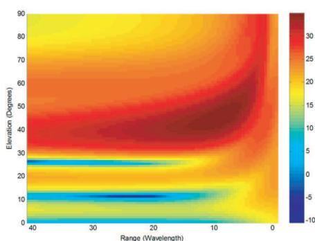
**Figure 7.** 3D transmit pattern slice at 50 degrees azimuth. Transmitter is focused at 45 degrees elevation and 50 degrees azimuth and 125 mm (10 wavelengths) range. Units in dB.
