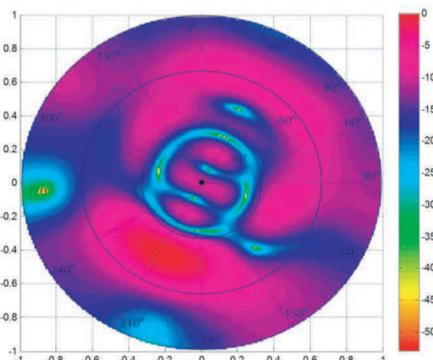
**Figure 11.** 2D transmit pattern projected onto unit circle. Power in dB relative to maximum beam power. Shows elevation null at  $20^\circ$  as well as beam at 210 degrees elevation and azimuth.
