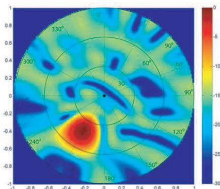
**Figure 8.** 2D transmit pattern projected onto unit circle. Power in dB. Negative range has been truncated to enhance beam visibility. For this pattern we have optimized the array pattern to provide a scanning beam at 210 degrees azimuth and 45 degrees elevation.
