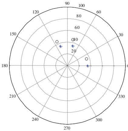
**Figure 12.** Two in sector near field and one out of sector long range target. Blue star indicates actual position of target. Circles indicate estimated position of target. All targets at 35 degrees elevation. Near field targets are at 75 and 114 degrees azimuth. Far field target at 0 degrees azimuth. All targets have equal amplitude. Near field targets are at range 10 wavelengths. Far field targets are at 50 wavelengths.
