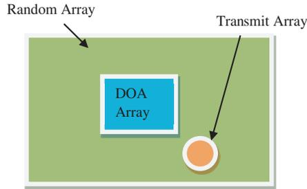
**Figure 1.** Array geometry — transmit array is a concentric circular array supporting MIMO usage. Central DOA array has elements arranged in regular rectangular grid. Random receive array supports imaging at close range.
