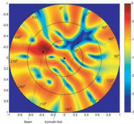
**Figure 10.** 2D transmit pattern projected onto unit circle. Power in dB relative to maximum beam power. This shows an azimuth null at 35 degrees extending from 15 to 65 degrees in elevation as well as the main beam at 45 degrees elevation and 300 degrees azimuth. Azimuth Null and beam direction can be seen.
