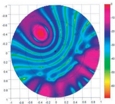
**Figure 6.** 3D transmit pattern slice at 125 mm range. Transmitter is focused at 45 degrees elevation and 320 degrees azimuth and 125 mm range. Units in dB.
