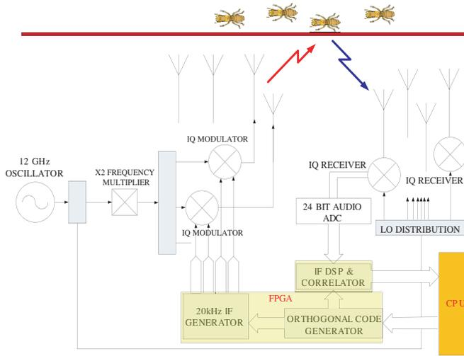
**Figure 3.** MIMO array block diagram-frequency up/down conversion performed via quadrature mixer with Tx array on left and Rx array on right. IF digitization via high resolution ADC with samples delivered to FPGA for initial processing. FPGA provides Rx & Tx control and MIMO processing. The CPU provides system control and user feedback.
