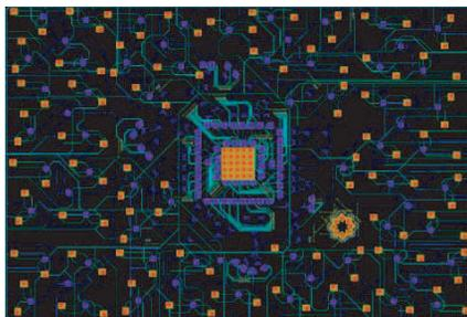
**Figure 2.** Hybrid array. Three distinct regions can be observed; a central dense receive array for far field use, a peripheral random receive array, and a small transmit array at lower right of the figure.
