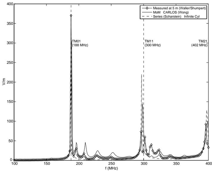
Figure 8. “Spatially averaged” internal fields, horizontal/ $TM$ .
