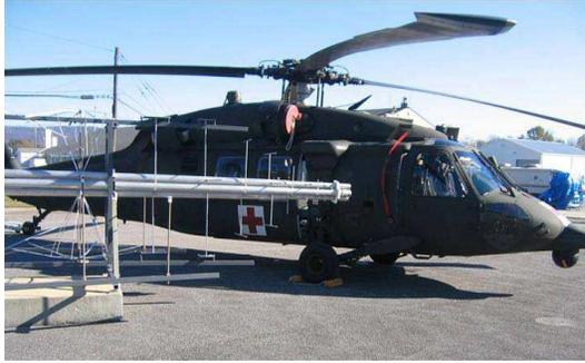
**Figure 11.** Typical EMV test setup.
