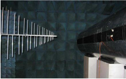
**Figure 1.** Measurement test setup on a 25 ft slotted circular cylinder.
