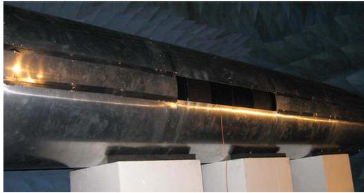
**Figure 12.** Measurement test setup on a 25 ft “shorted” slotted circular cylinder.
