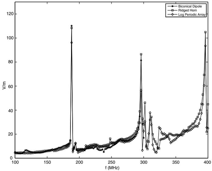
Figure 4. Measured aperture fields, horizontal/ $TM$ .
