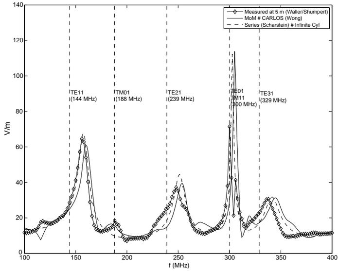
Figure 7. “Spatially averaged” internal fields, vertical/ $TE$ .
