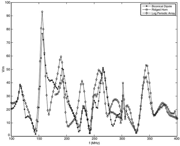
Figure 3. Measured aperture fields, vertical/ $TE$ .
