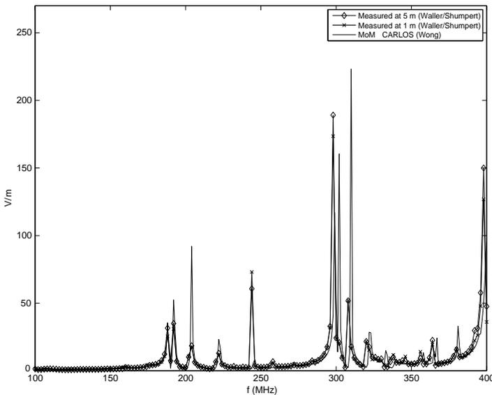
**Figure 14.** “Spatially averaged” internal fields, horizontal/*TM*, “shorted cylinder.”
