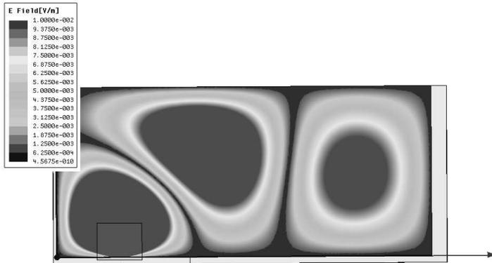
**Figure 8.** Coal ( $\sigma_{coal} = 10^{-6}$  S/m) panel section  $300\text{ m} \times 6\text{ m} \times 666.66\text{ m}$  fed from a  $20\text{ m} \times 1\text{ m}$  slot shaped waveport showing distorted  $TE_{102}$  mode field pattern and stored energy fields in the vicinity of the port. (Leaky case:  $\sigma_{coal} = 10^{-6}$  S/m;  $\sigma_{shale} = 1.0$  S/m).
