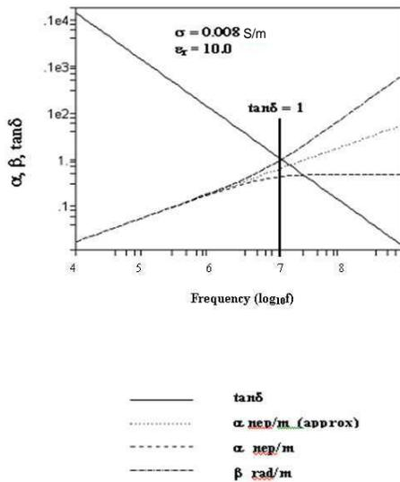
**Figure 2.** Propagation constants and loss tangent versus frequency for a UK coal medium having  $\sigma = 8.0 \text{ mS/m}$ ,  $\epsilon_r = 10$ ,  $\mu_r = 1$ .
