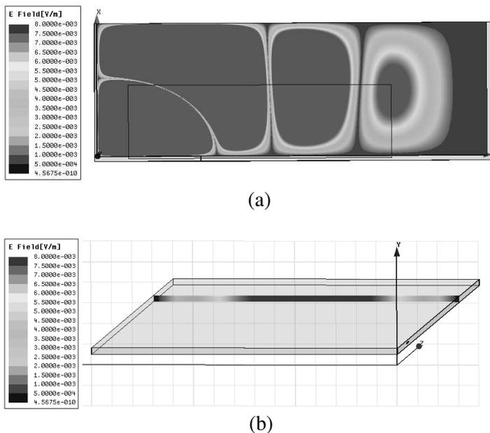
**Figure 7.** Coal ( $\sigma_{coal} = 10^{-4} \text{ S/m}$ ) panel section  $300 \text{ m} \times 6 \text{ m} \times 888.88 \text{ m}$  fed from a  $20 \text{ m} \times 1 \text{ m}$  slot shaped waveport showing  $TE_{10}$  mode field pattern (a) in  $x-z$  plane and (b) at a cross-sectional,  $x-y$  plane, located at  $z = 672 \text{ m}$ . (Lossy case:  $\sigma_{coal} = 0.0001 \text{ S/m}$ ;  $\sigma_{shale} = 10^5 \text{ S/m}$ ).
