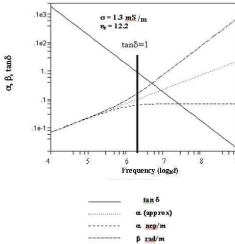
**Figure 1.** Propagation constants plus loss tangent versus frequency for a typical coal medium having  $\sigma = 1.3 \text{ mS/m}$ ,  $\epsilon_r = 12.2$ ,  $\mu_r = 1$ .
