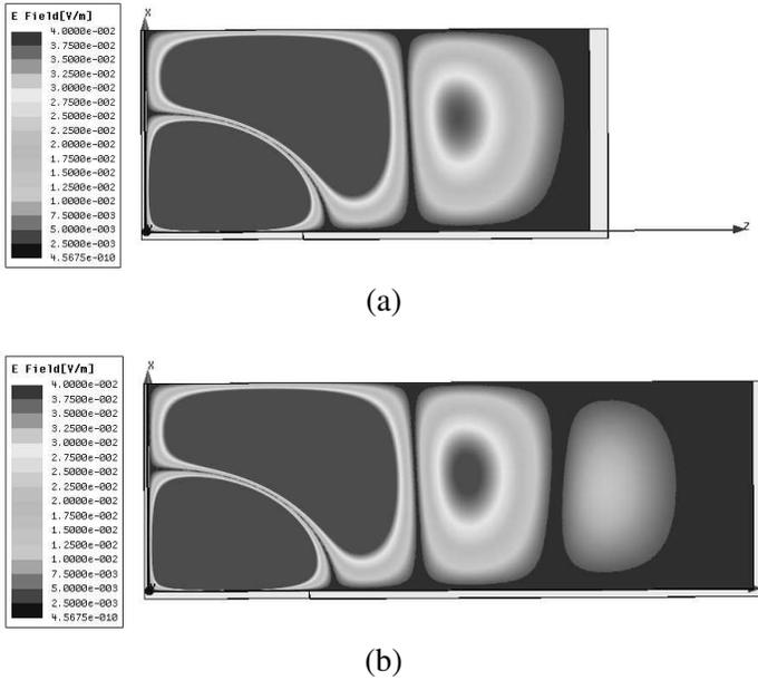
**Figure 6.** Coal ( $\sigma_{coal} = 10^{-4}$  S/m) panel section  $300 \text{ m} \times 6 \text{ m} \times L \text{ m}$  fed from a  $20 \text{ m} \times 1 \text{ m}$  slot shaped waveport showing the distorted TE<sub>10</sub> mode field pattern and stored energy fields in the vicinity of the port. The panel length in (a)  $L = 666.6 \text{ m}$ ; and in (b)  $L = 888.8 \text{ m}$  (Lossy case:  $\sigma_{coal} = 0.0001 \text{ S/m}$ ;  $\sigma_{shale} = 10^5 \text{ S/m}$ ).
