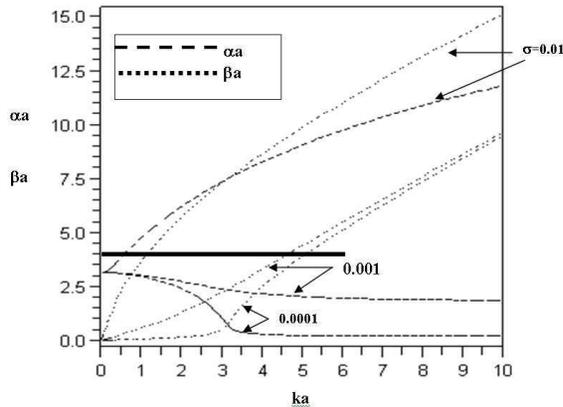
**Figure 3.** Brillouin diagram for  $TE_{10}$  modes in a coal-seam waveguide showing  $TE_{109}$  resonance frequencies in shorted waveguide ( $\epsilon_r = 10$ ,  $\mu_r = 1$ ). Note that in this figure  $\alpha \equiv \alpha_{10}$  and  $\beta \equiv \beta_{10}$ .
