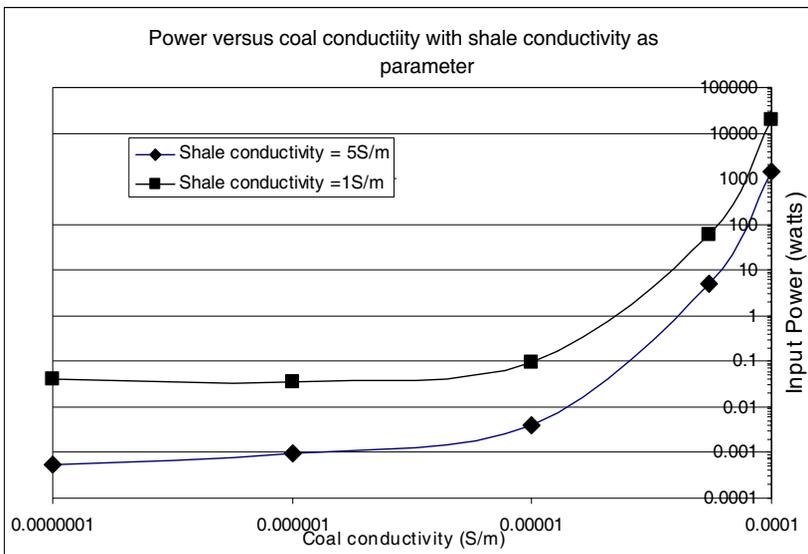
**Figure 10.** Injected power in watts to establish a  $E$ -field magnitude of 0.25 mV/m at 1000 m from input versus coal conductivity for 300 m wide by 6 m high coal panel, with shale conductivity as parameter. ( $\epsilon_{r-coal} = 10$ ;  $\epsilon_{r-shale} = 20$ ).
