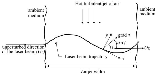
**Figure 2.** Local incidence angle  $i$  of the beam and refractive index gradient at any point  $M$  of the laser beam trajectory.  $\alpha = \text{angle}(\tau_0, \text{grad } n) = \text{angle}(Oz, \text{grad } n) \approx i$ .
