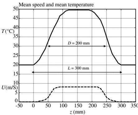
**Figure 3.** Definition of the jet width  $L = 300$  mm as the distance between the planes  $z = 0$  and  $z = L$  such that  $U(z = 0) = U(z = L) = 0$  and  $T(z = 0) = T(z = L) = \text{ambient temperature} = 20^\circ\text{C}$ .  $D = \text{width of the nozzle aperture} = 200$  mm.
