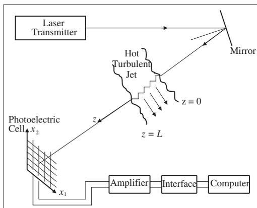
**Figure 1.** Experimental set-up [26, 29].
