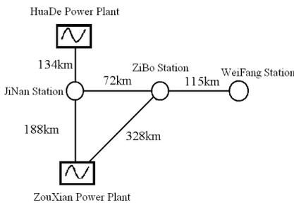
**Figure 2.** The associated 500 kV power network.
