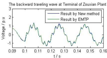
Figure 6. The waveform zooms in for closer image.
