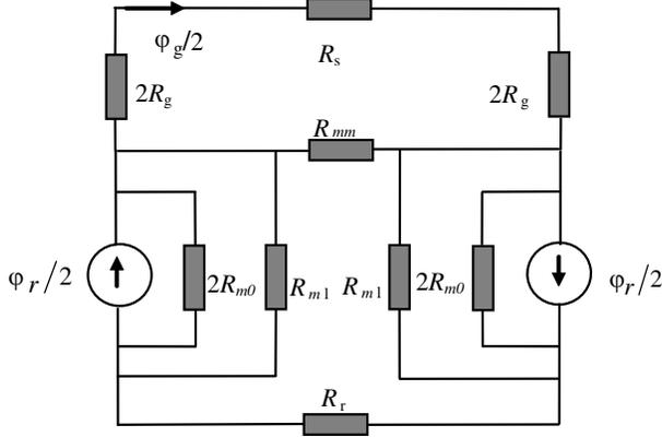
**Figure 2.** Magnetic circuit model of IPM synchronous motor.
