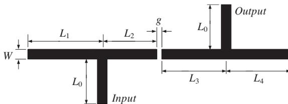
**Figure 3.** Microstrip bandpass filter: geometry [25].
