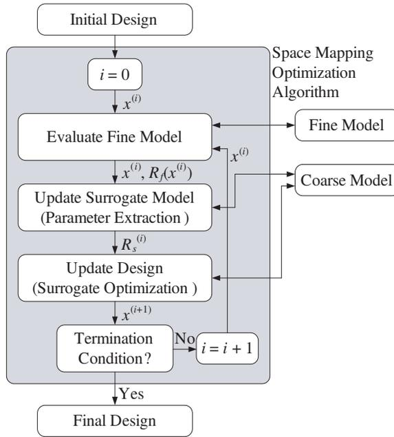
**Figure 1.** Flowchart of the space mapping algorithm. An approximate fine model optimum is obtained iteratively by optimizing the surrogate model. The fine model is evaluated at each new design for verification purposes. Parameter extraction and surrogate model optimization only involve coarse model.
