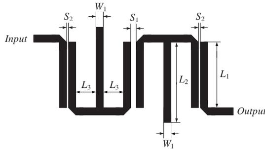
**Figure 5.** Geometry of the bandpass filter with open stub inverter [28].
