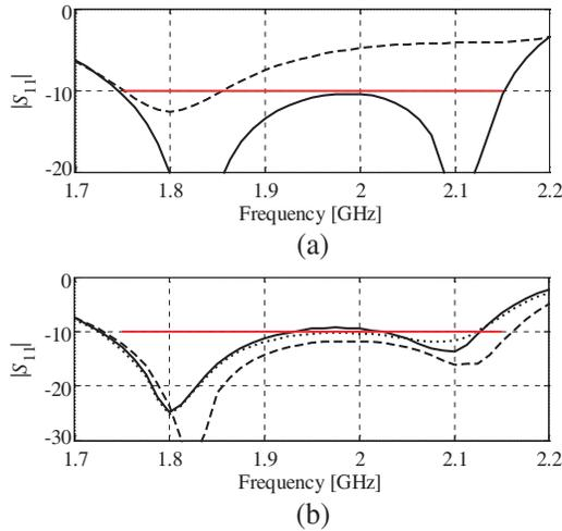
**Figure 10.** Double annular ring antenna: (a) Fine model response at the initial design (dashed line) and at the final design obtained using the SM algorithm presented here (solid line); (b) Fine model response at  $\mathbf{x}^{(0)}$  (solid line), and the coarse model at  $\mathbf{x}^{(0)}$  before (dashed line) and after (dotted line) parameter extraction.
