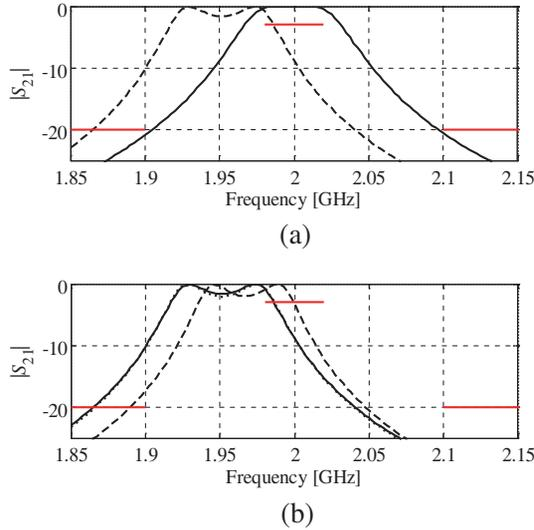
**Figure 6.** Microstrip bandpass filter: (a) Fine model response at the initial design (dashed line) and at the final design obtained using the SM algorithm presented here (solid line); (b) Fine model response at  $\mathbf{x}^{(0)}$  (solid line), and the coarse model at  $\mathbf{x}^{(0)}$  before (dashed line) and after (dotted line) parameter extraction.
