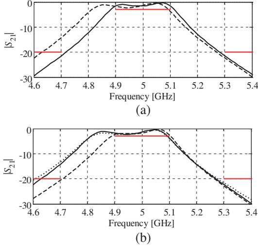
**Figure 4.** Microstrip bandpass filter: (a) Fine model response at the initial design (dashed line) and at the final design obtained using the SM algorithm presented here (solid line); (b) Fine model response at  $\mathbf{x}^{(0)}$  (solid line), and the coarse model at  $\mathbf{x}^{(0)}$  before (dashed line) and after (dotted line) parameter extraction.
