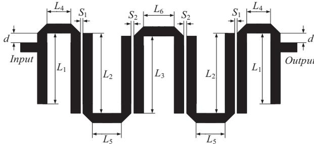
Figure 7. Microstrip hairpin filter: geometry [29].
