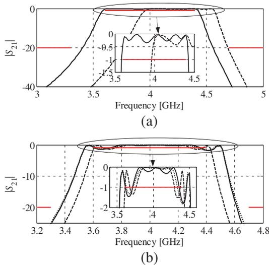
**Figure 8.** Hairpin filter: (a) Fine model response at the initial design (dashed line) and at the final design obtained using the SM algorithm presented here (solid line); (b) Fine model response at  $\mathbf{x}^{(0)}$  (solid line), and the coarse model at  $\mathbf{x}^{(0)}$  before (dashed line) and after (dotted line) parameter extraction.
