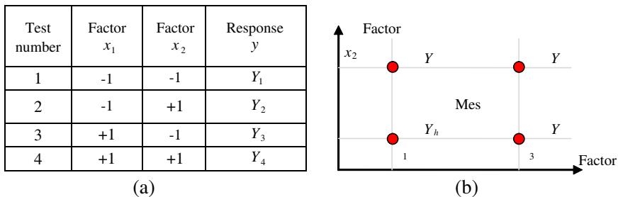
**Figure 4.** Full factorial design for 2 factors and 2 levels. (a) Design matrix. (b) Strategy of experimentation; points corresponding to nodes in the mesh of the experimental field.
