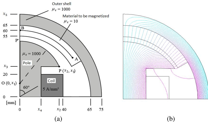
**Figure 5.** Magnetizer to be studied; (a) geometry, (b) contour of the solution.
