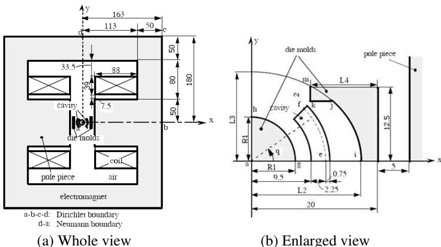
**Figure 9.** Model of die press with electromagnet.
