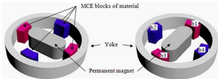
**Figure 12.** Configuration and operating principle of the PM cooling machine.
