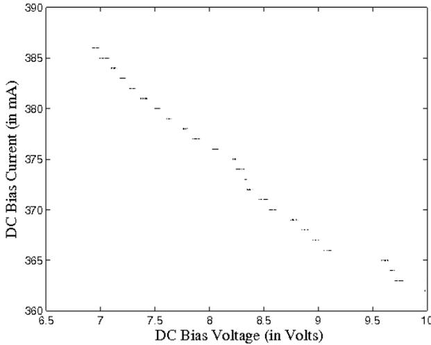
**Figure 2.** Experimentally obtained v-i characteristics of Gunn diode in negative resistance region.
