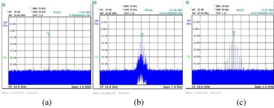
**Figure 11.** Output spectrum of the GO-2 in the BCGO system for three different states. Output powers and frequencies of GO-1 and GO-2 are respectively 14 dBm, 14.5 dBm, 10.012 GHz, 9.988 GHz.  $|k_{21}(\text{exp.})|$  is fixed at 0.187. (a) Synchronized state:  $|k_{12}(\text{exp.})| = 0.0398$ . (b) Chaotic state:  $|k_{12}(\text{exp.})| = 0.316$ . (c) Quasi-periodic state:  $|k_{12}(\text{exp.})| = 0.50$ .
