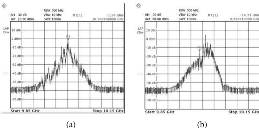
**Figure 10.** Selected output spectra of the GO-1 in the BCGO system: (a)  $|k_{12}(\text{exp.})| = 0.398$ ,  $|k_{21}(\text{exp.})| = 0.398$ ,  $f_1 = 10$  GHz,  $f_2 = 9.985$  GHz; (b)  $|k_{12}(\text{exp.})| = 0.398$ ,  $|k_{21}(\text{exp.})| = 0.630$ ,  $f_1 = 10$  GHz,  $f_2 = 10.007$  GHz.
