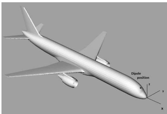
**Figure 10.** Boeing 757 fed with a vertical dipole.
