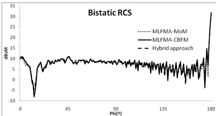
**Figure 9.** Bistatic RCS values at 36.0 GHz for the test case shown in Figure 8.
