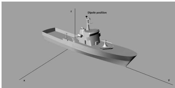
Figure 12. Ship fed with a vertical dipole.
