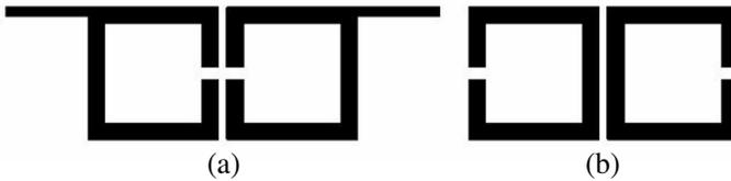
**Figure 15.** Proposed two-layered broadside-coupled filter. (a) Bottom layer, (b) top layer.
