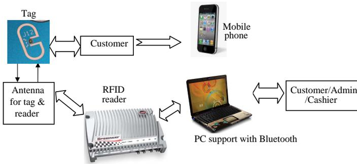
Figure 1. POS system using RFID and Bluetooth technology.
