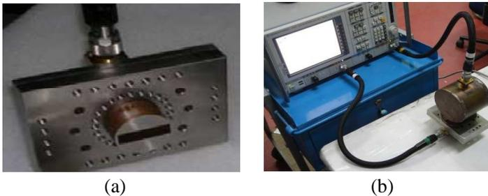
**Figure 7.** (a) Iris cylinder with rectangular iris. (b) Cavity connected to VNA through WR340-N Type adapter and auxiliary port for transmission measurements.
