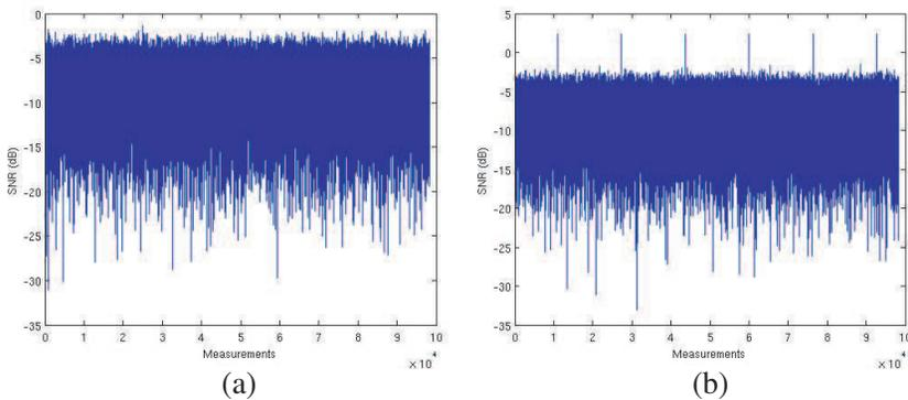
**Figure 4.** Sample observation sequence. (a) Clutter. (b) Target.
