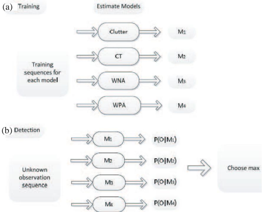
Figure 2. Using HMMs for target detection.
