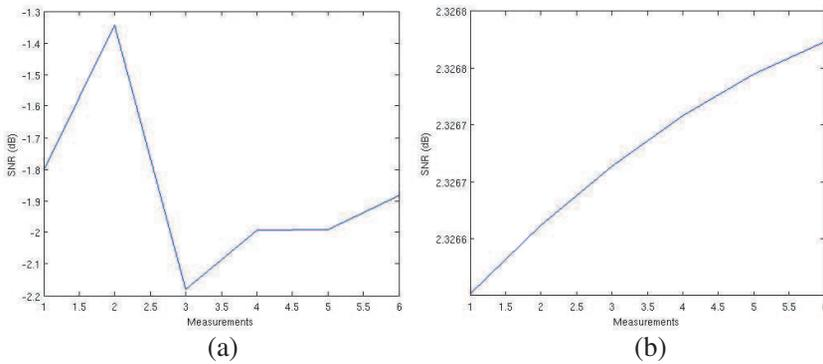
**Figure 5.** Variation of the signal power in a selected observation sequence. (a) Clutter. (b) Target.
