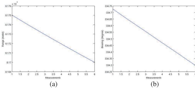
**Figure 6.** Range and bearing variation of the detected target. (a) Range. (b) Bearing.
