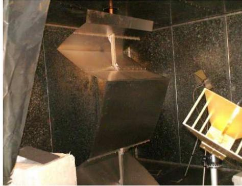
**Figure 2.** Inner view of the chamber. Foreground on the left, it is visible a part of a stirrer, then the sample under test on a support of foamed polystyrene. The other stirrer is visible on the center and the two double ridge antennas are on the right.
