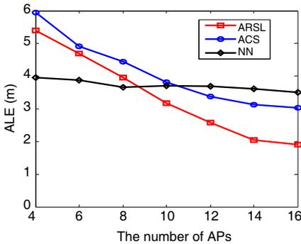
**Figure 5.** Effects of the number of APs on the localization error for targets from multiple categories.
