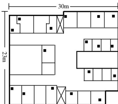
**Figure 1.** The configuration of localization area. The black dots show the locations of the APs.
