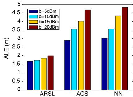
**Figure 6.** Robustness comparisons when RSS values are interfered by different fluctuation levels for targets from multiple categories.
