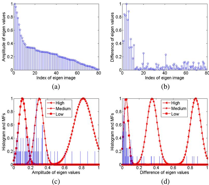
**Figure 2.** (a) Amplitude of eigen values of  $B$ -scan image. (b) Difference of eigen values. (c) MFs and histogram of eigen values. (d) MFs and histogram of difference of eigen values.
