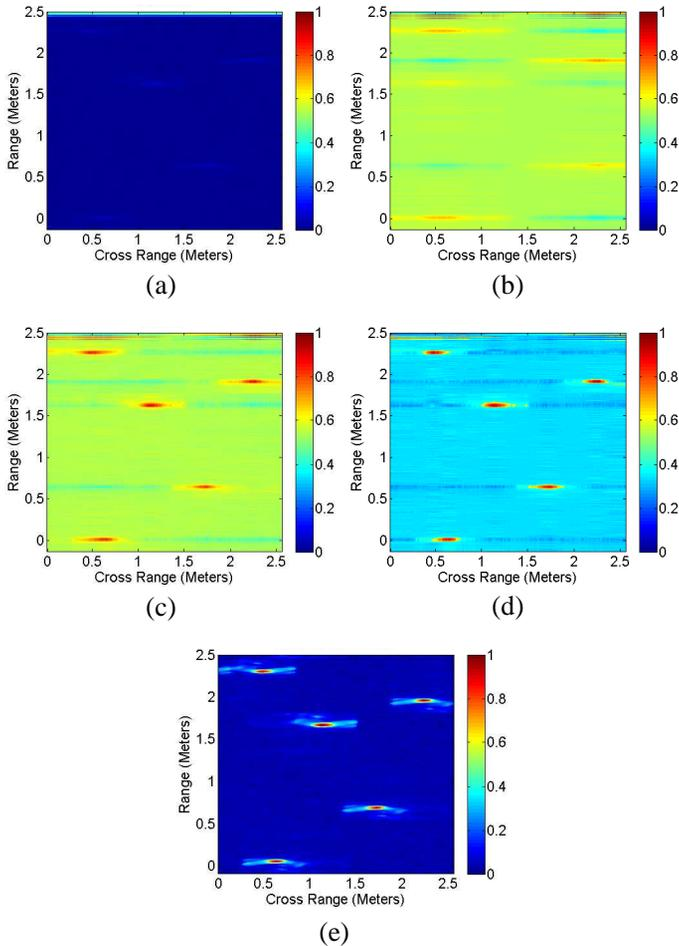
**Figure 7.** Images containing five targets. (a) Original *B*-scan image (b) Enhanced image using PCA [15]. (c) Enhanced image using FPCA [14]. (d) Enhanced image using proposed scheme. (e) Background subtracted image.
