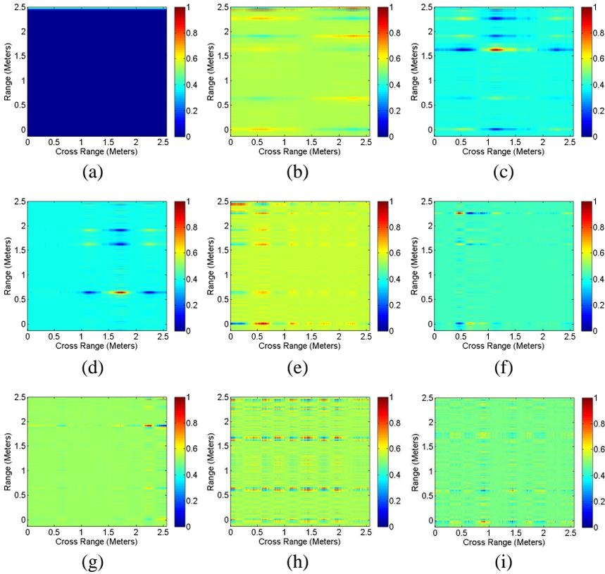
**Figure 5.** First nine eigen components of image containing five targets.
