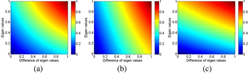
**Figure 3.** Output spectral weighting function Eq. (4): (a)  $\eta_1 = \eta_2 = 0.5$ , (b)  $\eta_1 = 0.25$  and  $\eta_2 = 0.75$ , (c)  $\eta_1 = 0.75$  and  $\eta_2 = 0.25$ .
