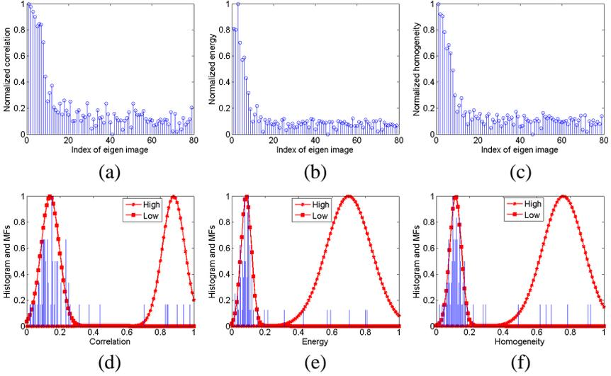
**Figure 4.** (a) Normalized correlation of eigen images. (b) Normalized energy of eigen images. (c) Normalized homogeneity of eigen images. (d) Histogram and MFs of correlation. (e) Histogram and MFs of energy. (d) Histogram and MFs of homogeneity.
