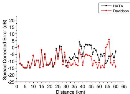
**Figure 12.** Spread corrected error along BODE-Sa'adu.
