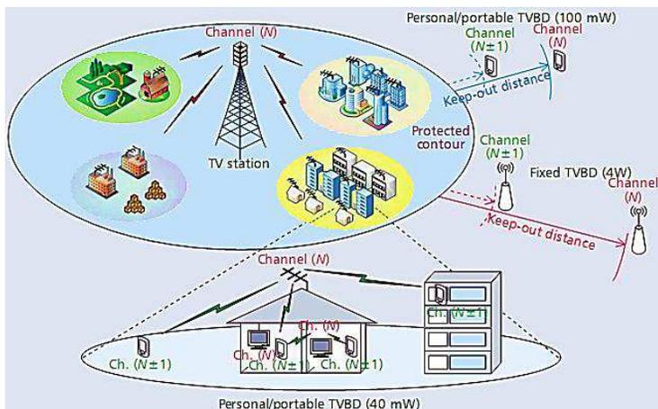
**Figure 1.** Deployment scenarios for co-channel and adjacent channel TV band devices in TV white space [2].
