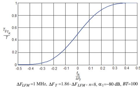
**Figure 4.** Dependency between time of group delay and frequency for a signal having a Taylor PSD function.
