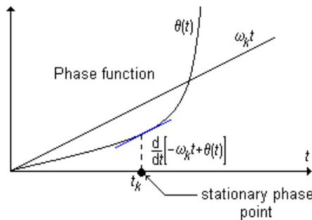
**Figure 1.** The criterion of stationary phase (the stationary point is achieved for  $t = t_k$  or  $\omega_k$ , when the tangent at function  $\theta(t)$  is parallel with straight line of  $\omega t$  etc.).
