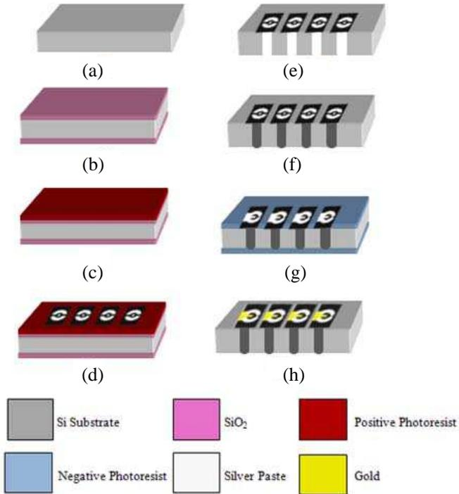
**Figure 2.** Fabrication process sequence for the vertical micro-coaxial transition. (a) Si substrate, (b) SiO<sub>2</sub> grown on the substrate, (c) photoresist deposited for patterning, (d) pattern transfer by photolithography, (e) removal of SiO<sub>2</sub> layer for etching and coaxial vias formed using deep reactive ion etching, (f) metallization of holes, (g) pattern transfer for CPW lines, and (i) CPW line metal deposition.
