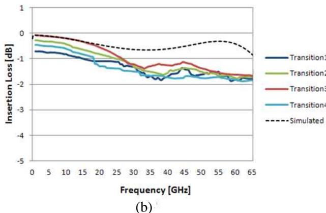
**Figure 8.** Measured results of micro-coaxial transition vs. simulated response with substrate integration. (a) Reflection coefficient and (b) insertion loss.
