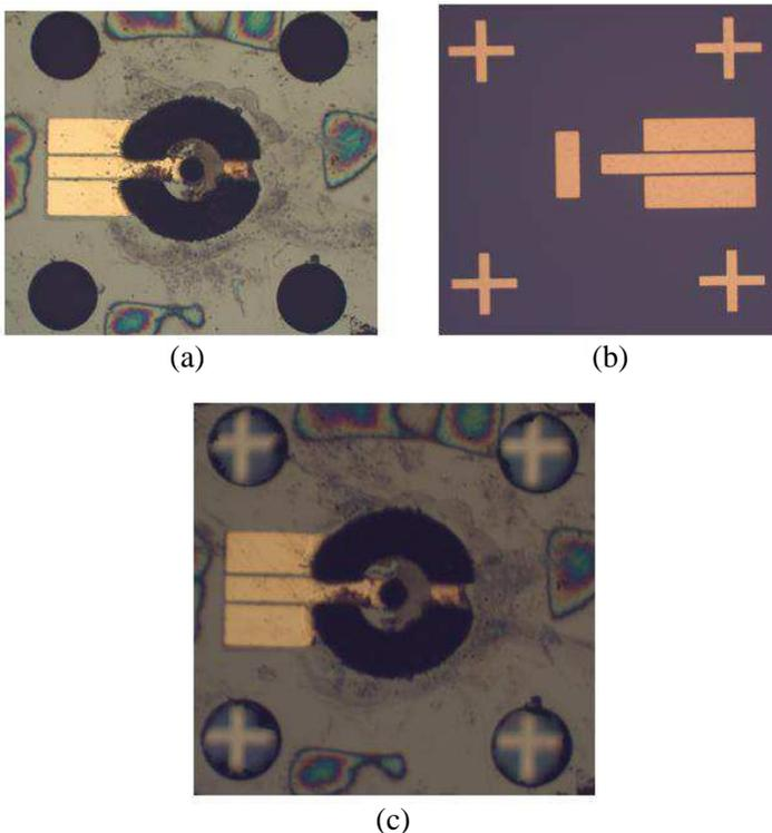
**Figure 7.** Microscopic images of fabricated micro-coaxial transition for integration. (a) Top substrate with etched local alignment holes, (b) additional substrate with cross hairs for extended CPW lines, and (c) substrate integration using local alignment holes and cross hairs.
