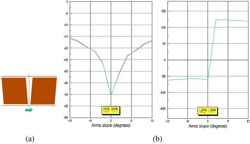
**Figure 8.** (a) Range of considered parallelograms with arms slope varying between  $-10^\circ$  and  $10^\circ$ ; (b) effect of the Parallelogram transformation on the magnitude and phase of the cross polarized components  $S_{xy}$  and  $S_{yx}$  of the scattering matrices.
