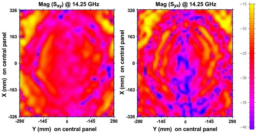
**Figure 16.** Magnitude of the Cross-polarization components  $S_{xy}$  and  $S_{yx}$  of the scattering matrices of the reflectarray elements of the central panel reconstructed from the measured radiation pattern (14.25 GHz).
