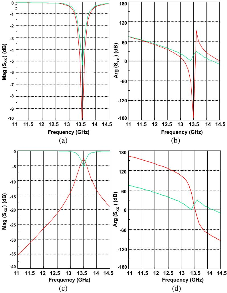
**Figure 15.** Scattering matrices of a reflectarray elements with a parasitic resonance (a) red:  $\text{Mag}(S_{xx})$ , green:  $\text{Mag}(S_{xx})$ , (b) red:  $\text{Arg}(S_{xx})$ , green:  $\text{Arg}(S_{xx})$ , (c) red:  $\text{Mag}(S_{xy})$ , green:  $\text{Mag}(S_{xx})$ , (d) red :  $\text{Arg}(S_{xy})$ , green:  $\text{Arg}(S_{xx})$ .
