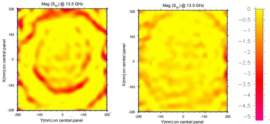
**Figure 14.** Magnitude of the Co-polarization components  $S_{xx}$  and  $S_{yy}$  of the scattering matrices of the reflectarray elements of the central panel reconstructed from the measured radiation pattern (13.5 GHz).
