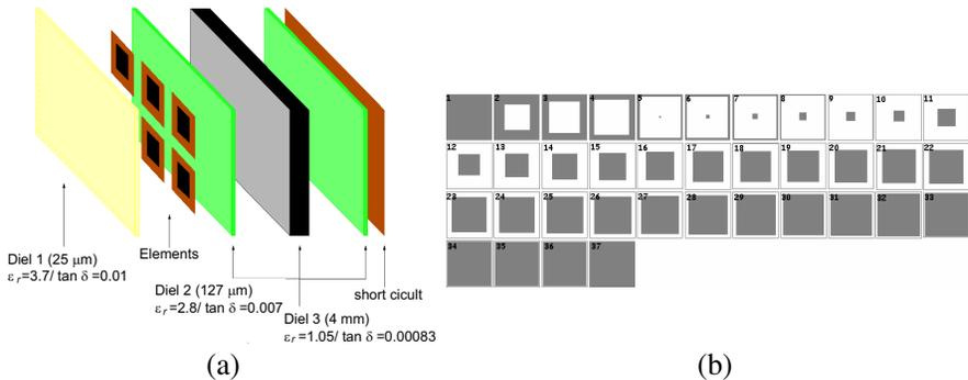
**Figure 3.** (a) Composite panel, (b) cycle of 37 Phoenix elements. One element is shown every  $10^\circ$ . Only the upper side of the elements is shown. Reflectarray lattice = 10.52 mm ( $0.5 \lambda$  at 14.25 GHz).
