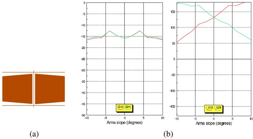
**Figure 9.** (a) Range of considered trapezoids with arms slope varying between  $-10^\circ$  and  $10^\circ$ ; (b) effect of the Trapezoid transformation on the magnitude and phase of the cross polarized components  $S_{xy}$  and  $S_{yx}$  of the scattering matrices.
