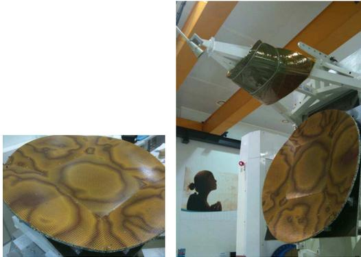
**Figure 11.** The 1.3m assembled reflectarray made of five inclined panels.
