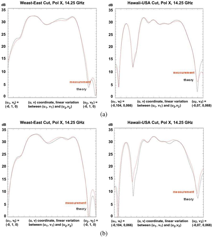
**Figure 13.** Comparison of the simulated (black lines) and measured (red lines) radiation patterns (a) in polarization  $X$  and (b) in polarization  $Y$ , 14.25 GHz. East-West Cuts and a diagonal cut through Hawaii and USA.
