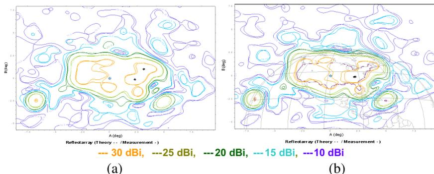
**Figure 12.** Comparison of the simulated (dotted lines) and measured (plain lines) radiation patterns (a) in polarization  $X$  and (b) in polarization  $Y$ , 14.25 GHz.
