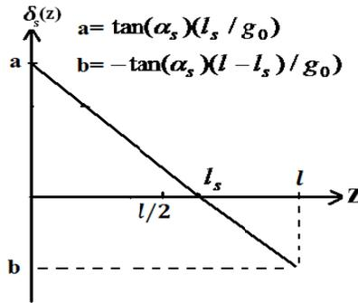
**Figure 3.** Variation of static eccentricity coefficient in different positions for machine under static misalignment.
