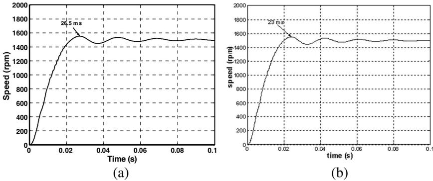
**Figure 11.** Motor speed from (a) simulation under healthy and (b) misalignment conditions.
