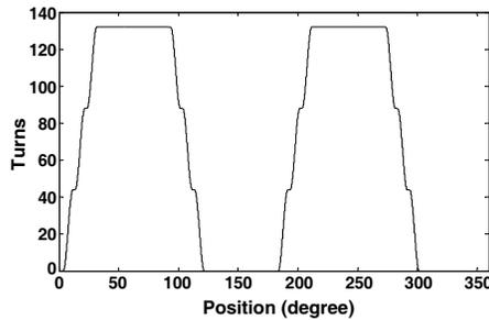
**Figure 1.** Turn function of the stator phase A.
