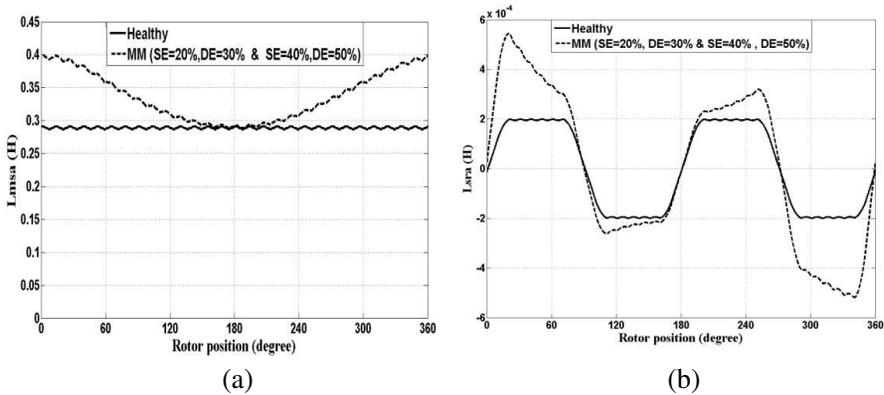
**Figure 10.** Magnetizing inductance of (a) stator phase *A* and (b) mutual inductance between stator phase *A* and rotor loop 1, as a function of rotor position under healthy and mixed rotor misalignment conditions.
