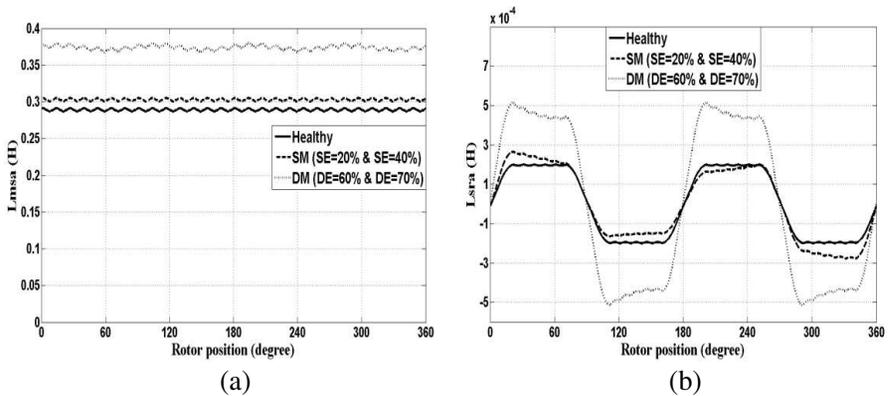
**Figure 9.** Magnetizing inductance of (a) stator phase *A* and (b) mutual inductance between phase *A* and rotor loop 1, as a function of rotor position under healthy, static and dynamic rotor misalignment conditions.
