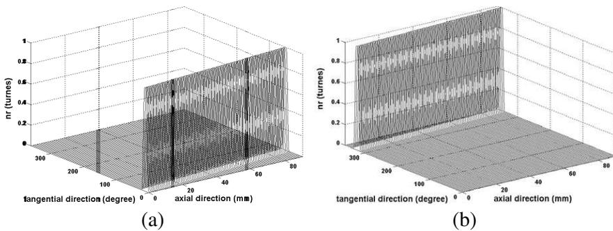
**Figure 7.** Turn function of (a) the rotor loop 1 and (b) rotor loop 28, considering skew effect.
