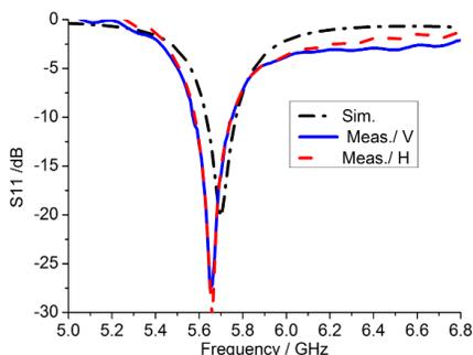
**Figure 17.** Simulated and measured  $S_{11}$  of the LPs.
