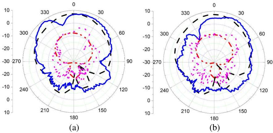
**Figure 11.** Simulated and measured  $E$ -plane pattern for the LP operations at 5.78 GHz. --- Co-Pol/Sim., — Co-Pol/Meas., -·-·- X-Pol/Sim., ..... X-Pol/Meas.. (a) H-port; (b) V-port.
