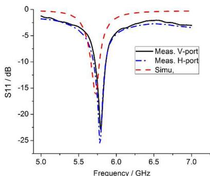
**Figure 9.** Measured  $S_{11}$  of the linear polarization states.
