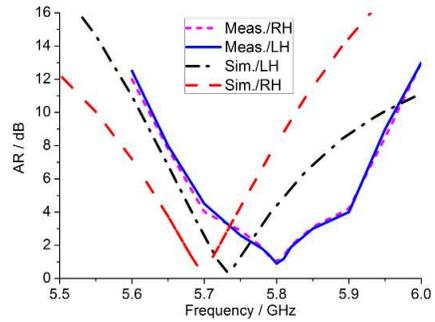
**Figure 21.** Simulated and measured AR for the CPs.
