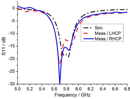
**Figure 20.** Measured  $S_{11}$  of the CP operations.
