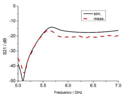
**Figure 18.** Simulated and measured  $S_{21}$  of the LPs.
