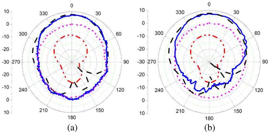
**Figure 19.** Simulated and measured co- and cross-polarization patterns for the LP operations at 5.66 GHz. --- Co-Pol/Sim., - - - - Co-Pol/Meas., - · · · X-Pol/Sim., ····· X-Pol/Meas.. (a) H-port; (b) V-port.
