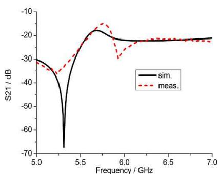
**Figure 10.** Measured  $S_{21}$  of the linear polarization states.
