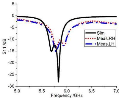
**Figure 12.** Simulated and measured  $S_{11}$  of the CPs.
