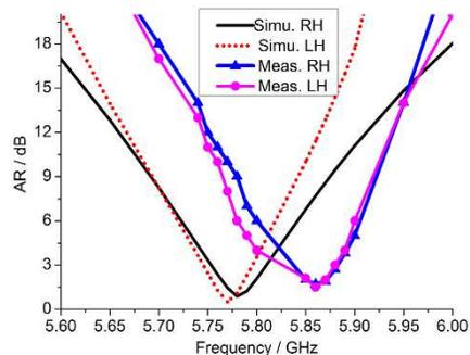
**Figure 13.** Simulated and measured AR of the CPs.
