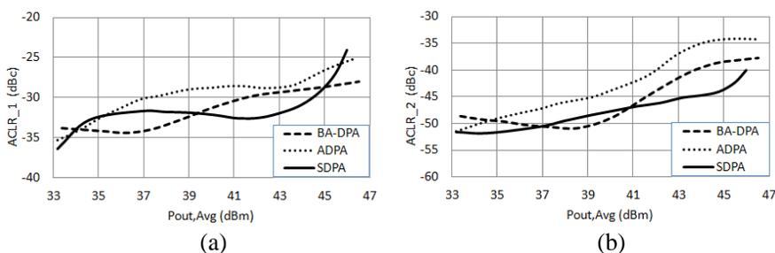
**Figure 10.** Measured Linearity characteristics of of Asymmetric DPA (ADPA) and Bias Adapted-DPA (BA-DPA) in Comparison to Symmetrical DPA (SDPA); W-CDMA signal with PAPR = 6.5 dB. (a) ACLR<sub>1</sub> (5 MHz offset). (b) ACLR<sub>2</sub> (10 MHz offset).
