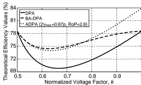
**Figure 4.** Theoretical efficiency characteristic of asymmetrical DPA (ADPA) with  $2 \cdot \gamma_{\max} = 0.67\pi$  and RoP = 2.6 in comparison to bias adapted-DPA (BA-DPA) and ideal class-B/class-B DPA.
