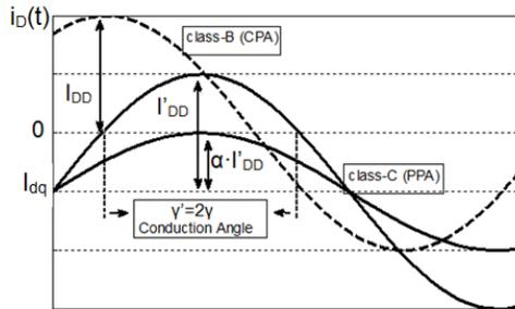
**Figure 2.** Drain current waveforms of CPA and PPA.
