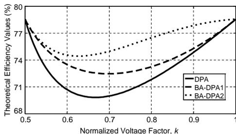
**Figure 3.** Theoretical efficiency characteristics in load modulation region (DPA: ideal, class-B/class-B DPA, BA-DPA1: linearly changing gate voltage adaptation, BA-DPA2: linearly changing conduction angle adaptation).
