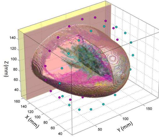
**Figure 1.** MRI-derived FDTD model and antennas setup.
