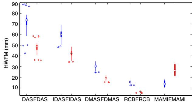
**Figure 6.** Half Width Full Maximum: box plot over 25 samples for non-filtered (blue) and pre-filtered (red) beamformers.
