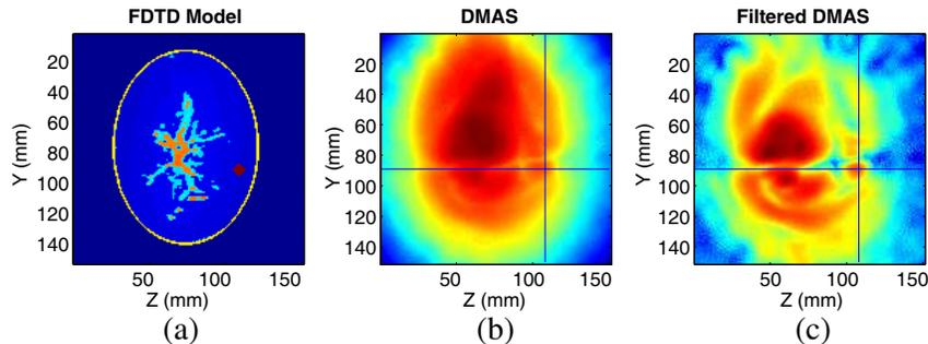
**Figure 7.** Effects of pre-filtering on the DMAS beamformer applied to a dense dielectrically-heterogeneous breast. While tumour detection is very difficult in such scenarios, the presence and location of the tumour only becomes discernible when pre-filtering is applied.
