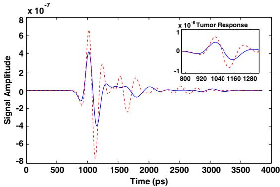
**Figure 3.** A sample received signal ( $S_{(1,6)}$  (solid blue), transmitted from antenna 1 and received at antenna 6) with the corresponding filtered signal shown in red. The pre-filtering process compensates for path-dependent dispersion effects. The scaled tumour response is also shown inset.
