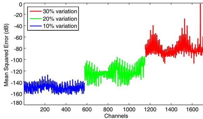
**Figure 8.** Effect of pre-filtering: Mean Squared Error (MSE) of filtered signals and simulated non-dispersive signals on three MRI-derived numerical breast models; (BLUE) A model with less than 10% variation in average dielectric properties; (GREEN) model with 20% variation; (RED) model with 30% variation in average dielectric properties.
