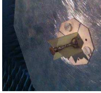
Figure 6. Prototype of the sensor A on a metallic plate of 300 mm in diameter.
