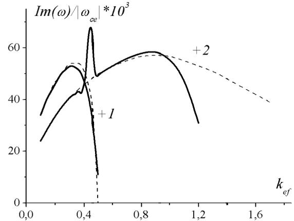
**Figure 3.** The growth rate of the ASW resonance beam instability as a function of the effective wave number for the different values of the azimuthal mode numbers. The parameters of the beam-plasma system are the same as in Figure 2.
