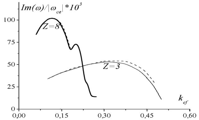
**Figure 5.** The growth rate of the ASW resonance beam instability as a function of the effective wave number for different values of the external magnetic field. The parameters of the beam-plasma system are the same as in Figure 4.
