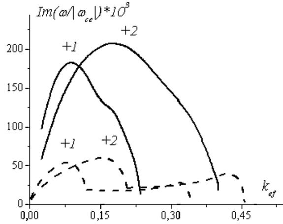
**Figure 8.** The growth rate of the ASW resonance beam instability as a function of the effective wave number for different beam densities.  $Z = 10$ ,  $\Delta = 0.2$ . Solid lines correspond to strong beam,  $\alpha = 10^{-2}$ , dashed lines — weak beam,  $\alpha = 10^{-4}$ .
