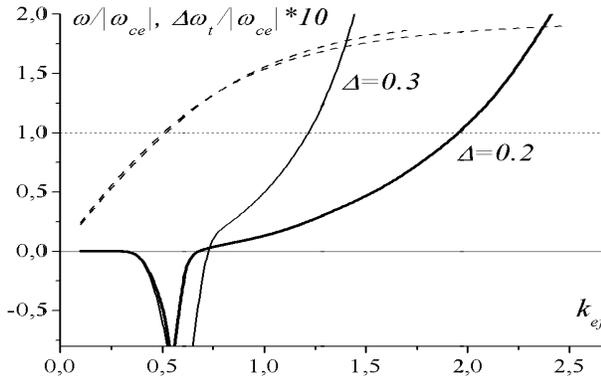
**Figure 6.** The correction to the ASW frequency caused by the toroidicity of the external magnetic field as a function of the effective wave number for different widths of the vacuum gap;  $m = +2$ ;  $Z = 3$ . In case of  $\Delta = 0.3$ , the parameter of toroidicity  $\varepsilon_t = 0.1$ , in case of  $\Delta = 0.2$ , the parameter of toroidicity  $\varepsilon_t = 0.05$ .
