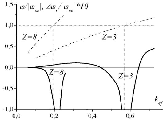
**Figure 4.** The correction to the ASW frequency caused by the toroidicity of the external magnetic field as a function of the effective wave number for different values of the external magnetic fields;  $m = +1$ ;  $\Delta = 0.3$ ;  $\varepsilon_t = 0.1$ .
