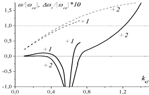
**Figure 2.** Correction to the ASW frequency caused by the toroidicity of the external magnetic field as a function of the effective wave number for different azimuthal mode numbers. The numbers correspond to the values of  $m$ ;  $Z = 3$ ;  $\Delta = 0.3$ ;  $\varepsilon_t = 0.1$ .
