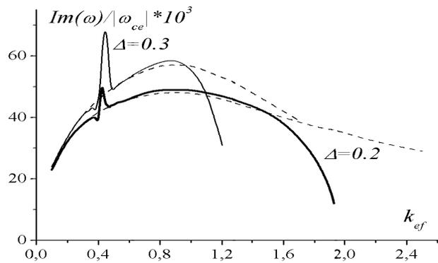
**Figure 7.** The growth rate of the ASW resonance beam instability as a function of the effective wave number for different widths of the vacuum gap. The parameters of the beam-plasma system are the same as in Figure 6.
