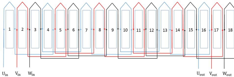
Figure 3. Winding pattern for three-phase 18-slot motor.
