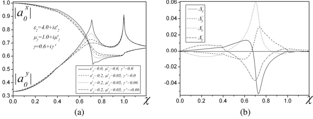
**Figure 5.** The frequency dependence of the (a) reflection coefficients and (b)  $\Delta_{x,y}^\pm$  coefficients in the presence of losses, the case of the incidence of right-handed circularly polarized wave ( $d/l = 0.5$ ,  $\varepsilon_1 = 1$ ,  $\mu_1 = 1$ ).
