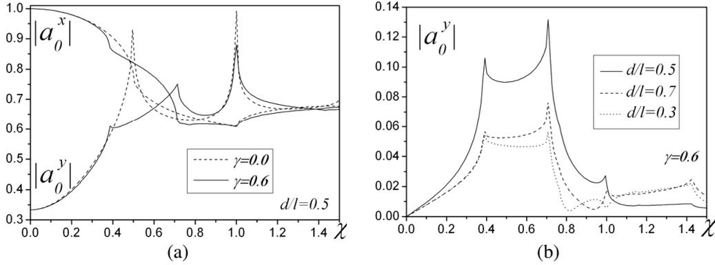
**Figure 2.** The reflection coefficients of the (a) co- and (b) cross-polarized waves as a function of the frequency parameter  $\chi$  for  $E$ - and for  $H$ -incident waves ( $\varepsilon_1 = 1$ ,  $\mu_1 = 1$ ,  $\varepsilon_2 = 4$ ,  $\mu_2 = 1$ ).
