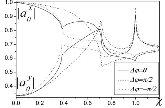
**Figure 4.** The frequency dependences of the reflection coefficients at simultaneous incidence of  $E$ - and  $H$ -waves ( $d/l = 0.5$ ,  $\varepsilon_1 = 1$ ,  $\mu_1 = 1$ ,  $\varepsilon_2 = 4$ ,  $\mu_2 = 1$ ,  $\gamma = 0.6$ ).
