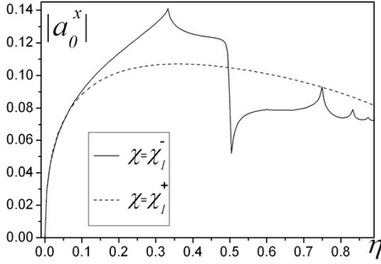
**Figure 3.** The reflection coefficient of the cross-polarized wave versus the relative chirality parameter  $\eta$ , ( $\chi = \chi_1^\pm$ ,  $d/l = 0.5$ ,  $\varepsilon_1 = 1$ ,  $\mu_1 = 1$ ,  $\varepsilon_2 = 4$ ,  $\mu_2 = 1$ ).
