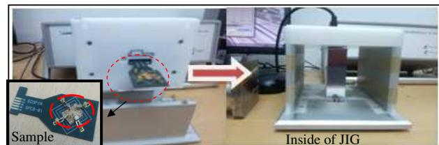
Figure 7. Sample PB board placement inside of jig.
