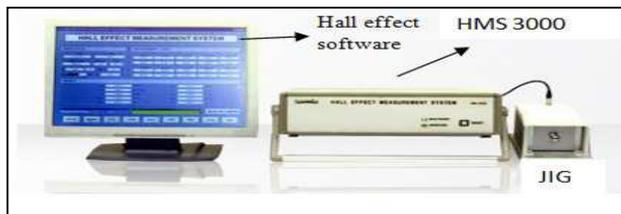
Figure 6. Hall effect measurement HMS 3000 setup.
