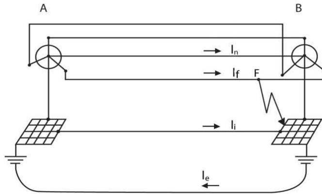
**Figure 1.** Main parts of the ground fault current.
