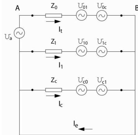
**Figure 4.** Equivalent circuit of the introduced line model.
