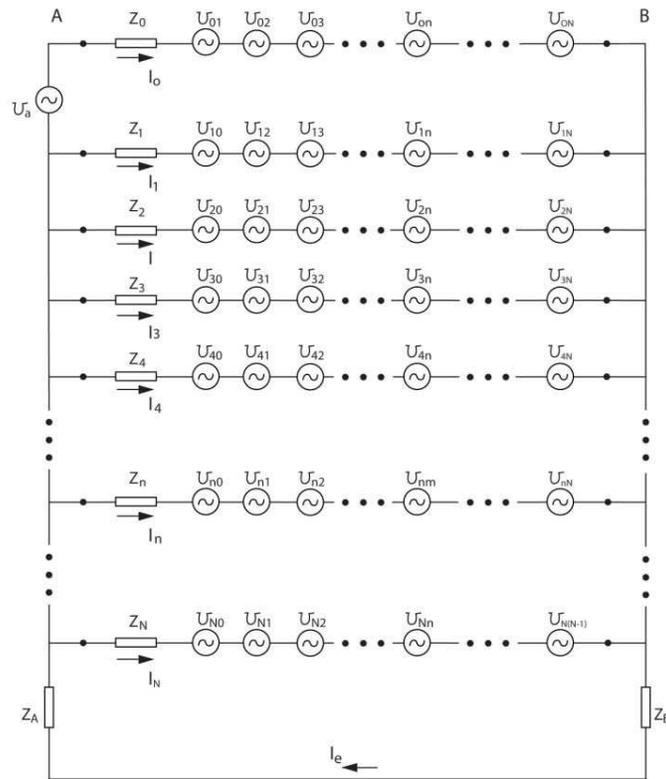
**Figure 2.** The complete line equivalent circuit.
