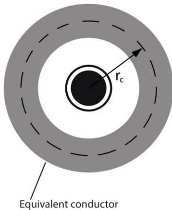
**Figure 3.** Cross section of the introduced line model.
